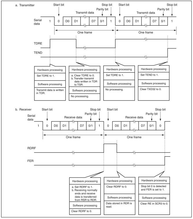
Figure 3.1 Operation Principle of Simultaneous Serial Data Transmission and Reception in Asynchronous Mode
