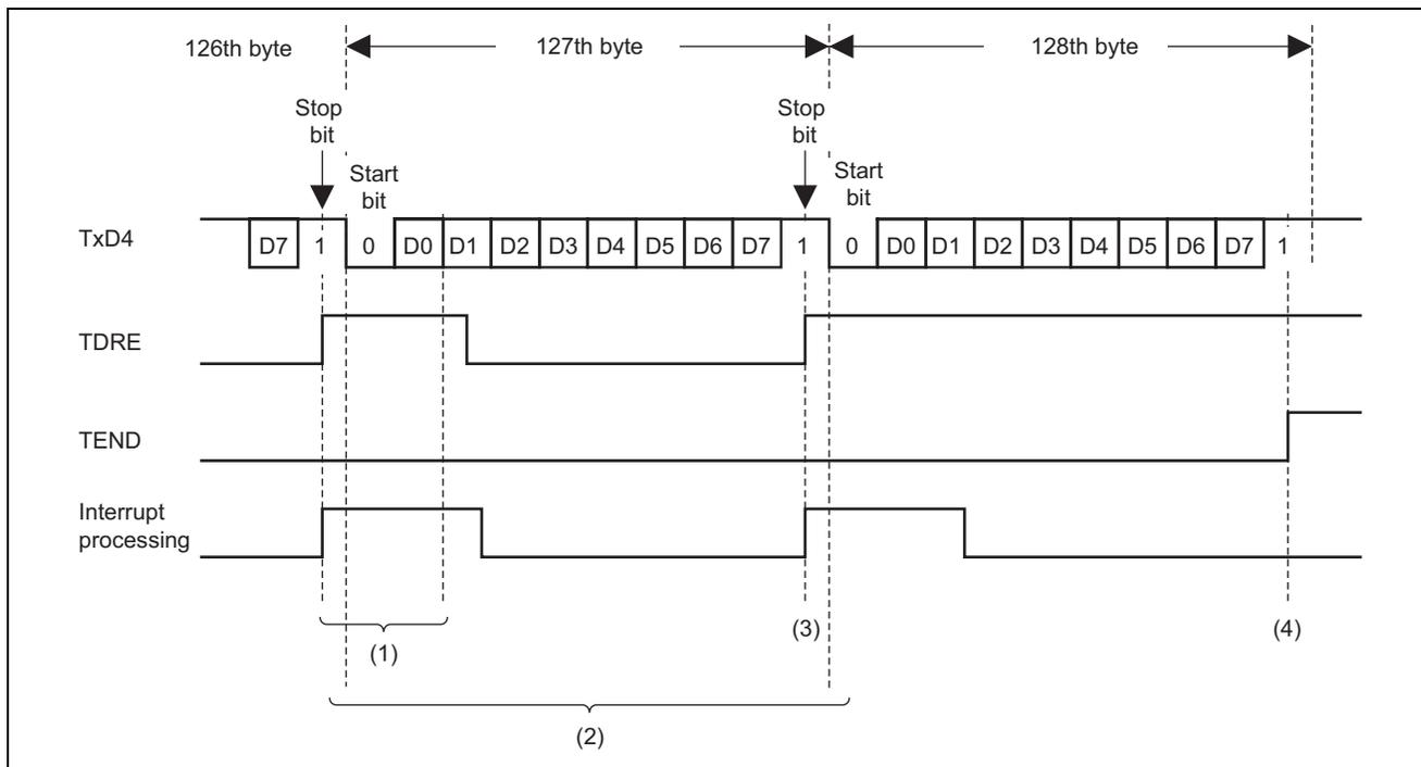
**Figure 4 Transmit Operation Timing**
