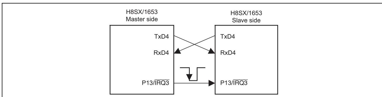
**Figure 1 Connection for Simultaneous Transmission and Reception by SCI in Asynchronous Mode**
