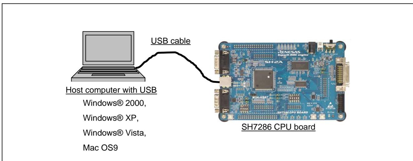
**Figure 1 System Configuration**
