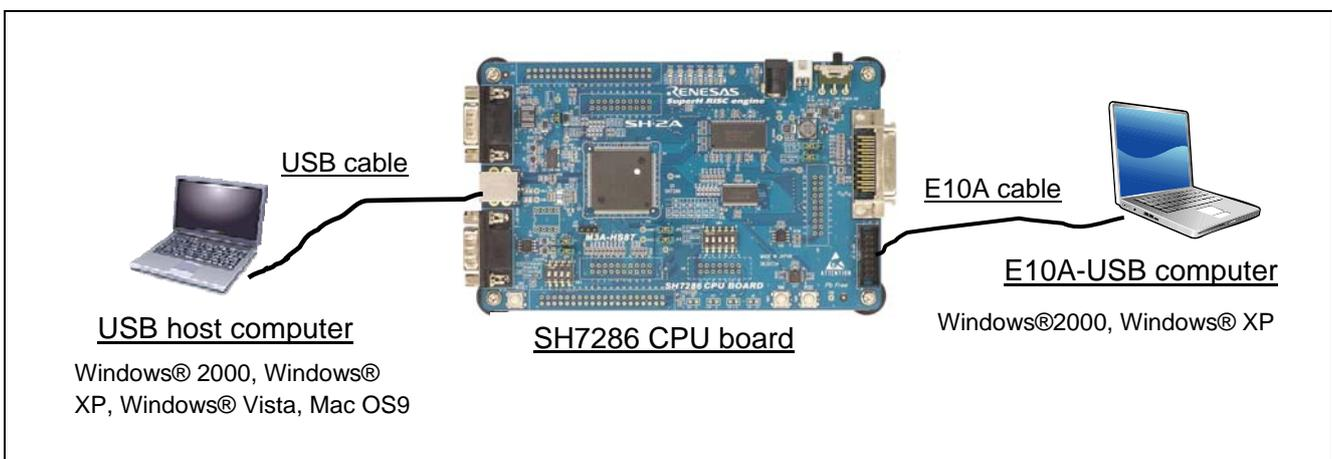
**Figure 3 Device Connection Diagram**
