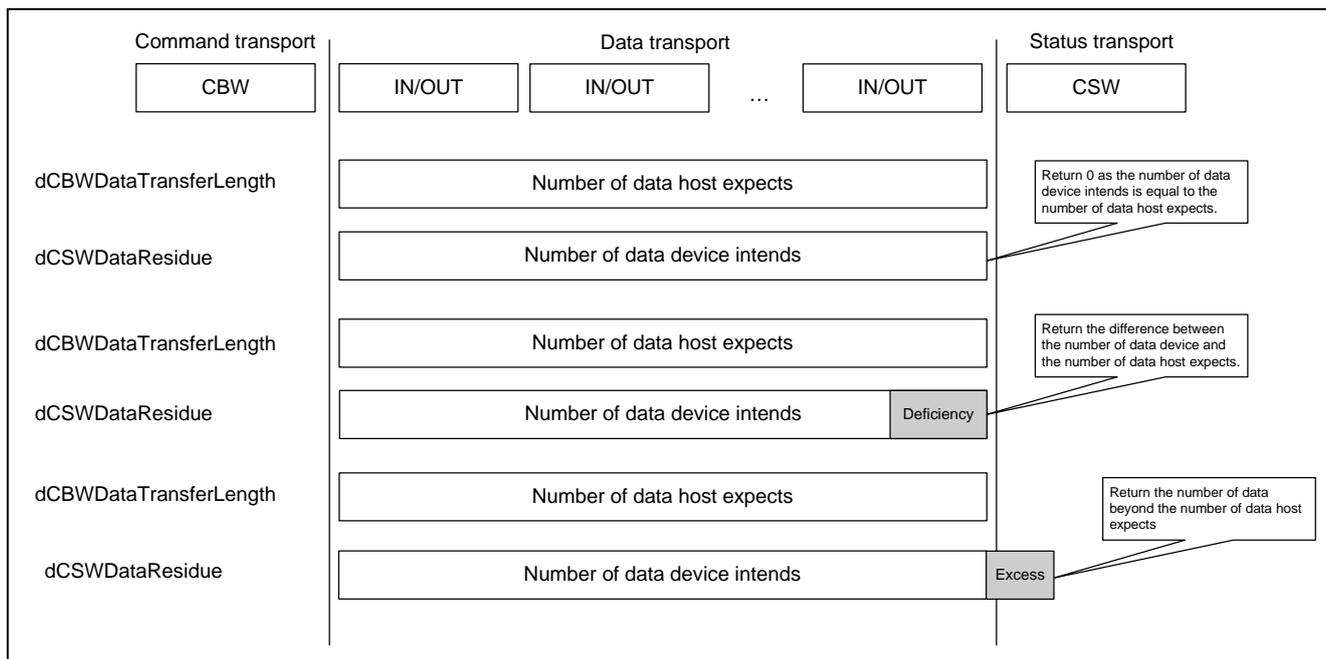
Figure 11 Stages on Bulk-Only Transport
