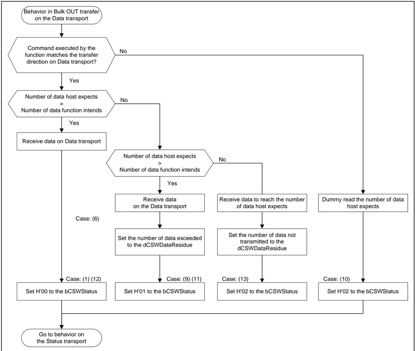
Figure 10 Flow Chart for Error Handling on Data Transfer (3/3)
