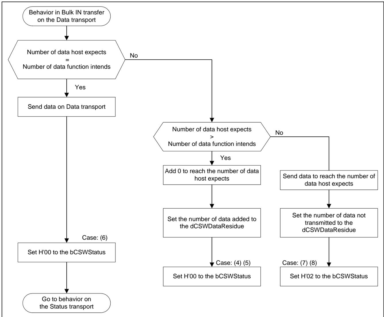
Figure 9 Flow Chart for Error Handling on Data Transfer (2/3)
