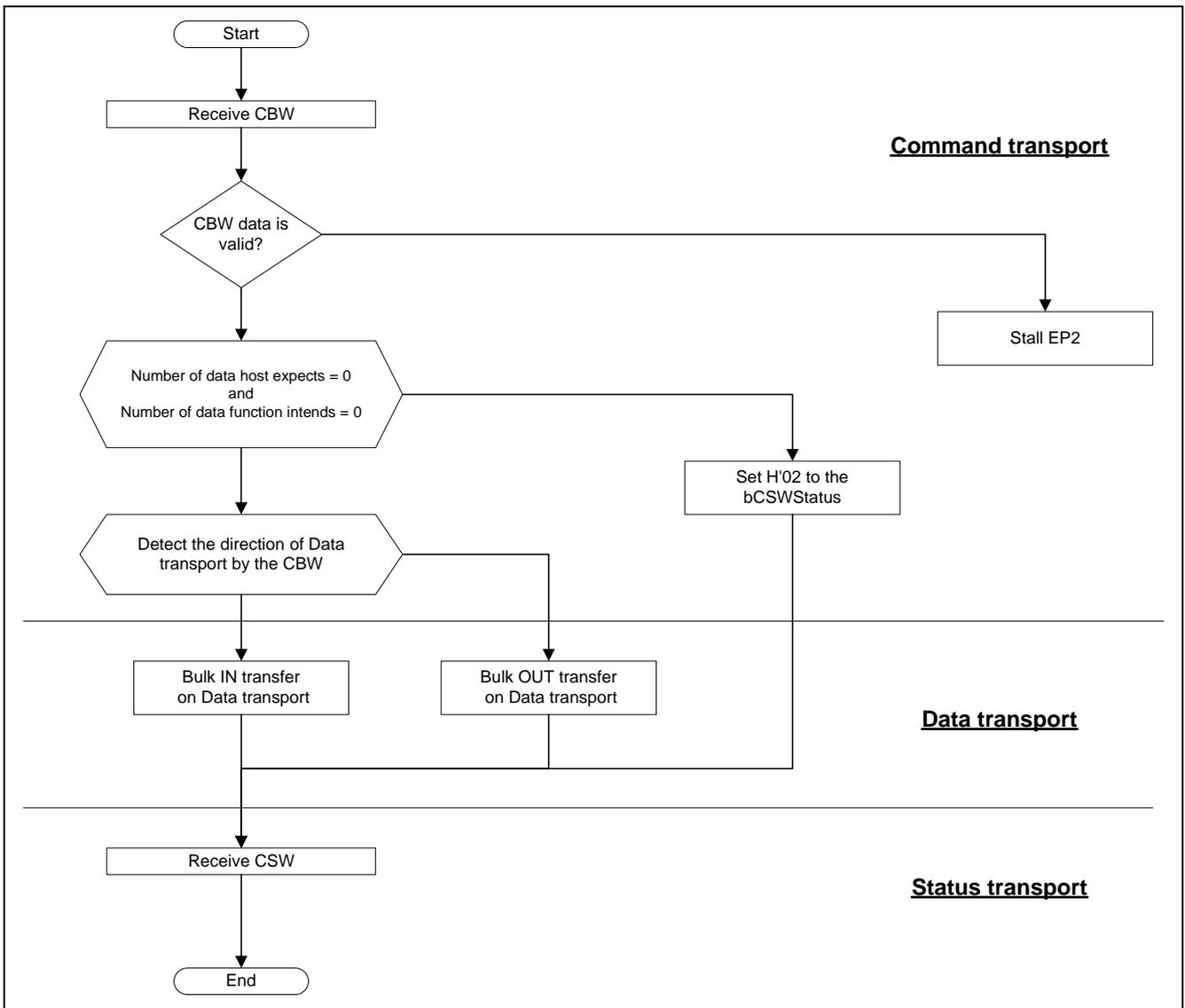
Figure 8 Flow Chart for Error Handling on Data Transfer (1/3)
