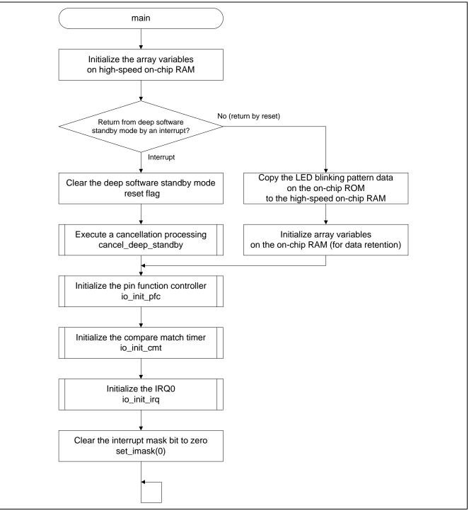
Figure 6.2 Procedure of Main Processing
