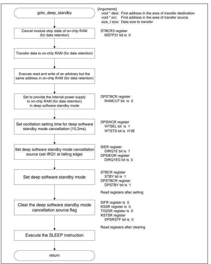
Figure 6.6 Procedure of Transition Processing to Deep Software Standby Mode
