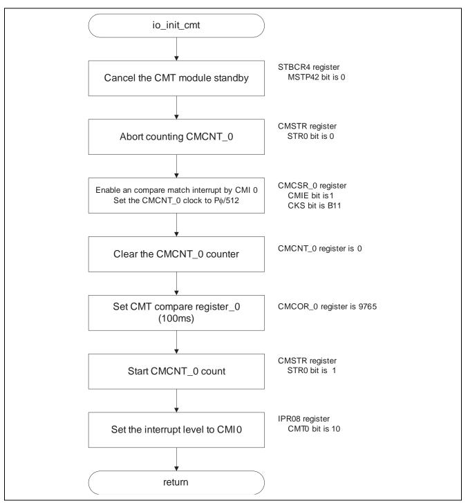
Figure 6.4 Procedure of Initial Setting for Compare Match Timer
