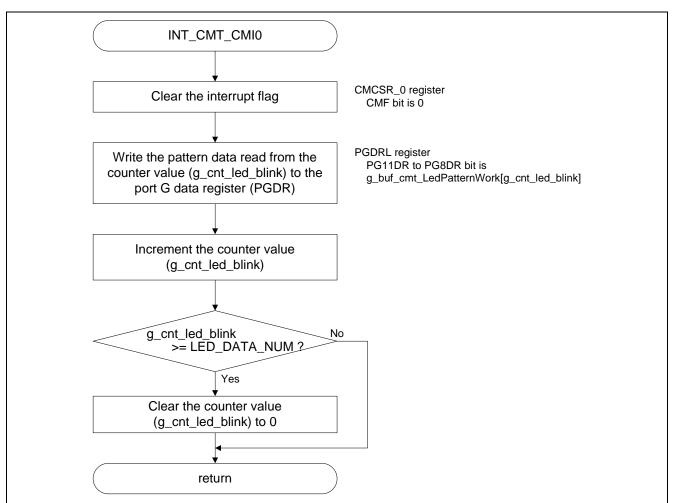
Figure 6.9 Procedure of CMI0 Interrupt Processing
