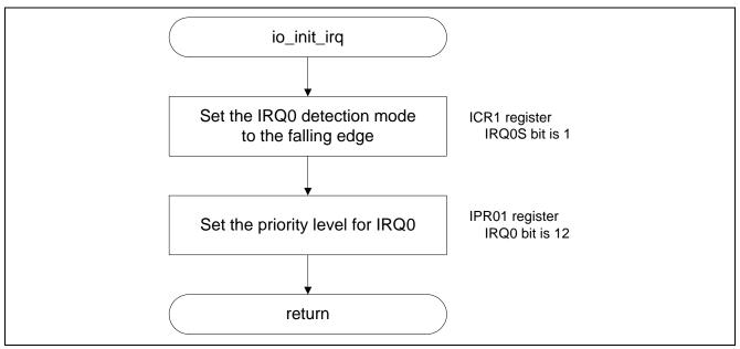
Figure 6.5 Procedure of Initial Setting for IRQ
