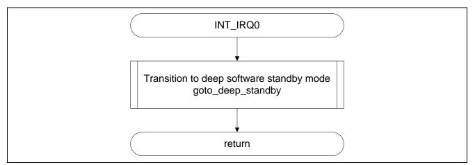
Figure 6.8 Procedure of IRQ0 Interrupt Processing (Transition to Deep Software standby Mode)
