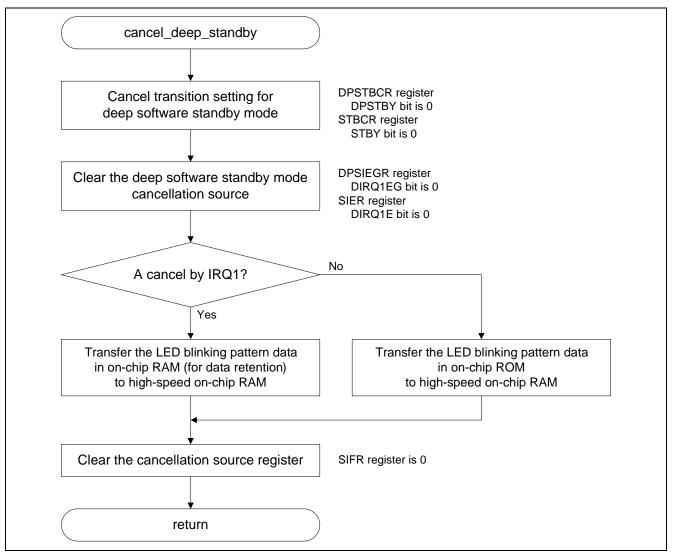
Figure 6.7 Procedure of Return Processing from Deep Software Standby Mode
