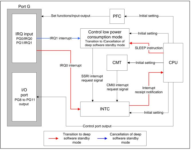
Figure 1.1 Block Diagram of Peripheral Functions
