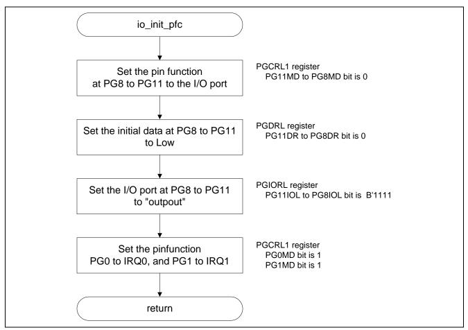
Figure 6.3 Procedure of Initial Setting for Pin Function Controller
