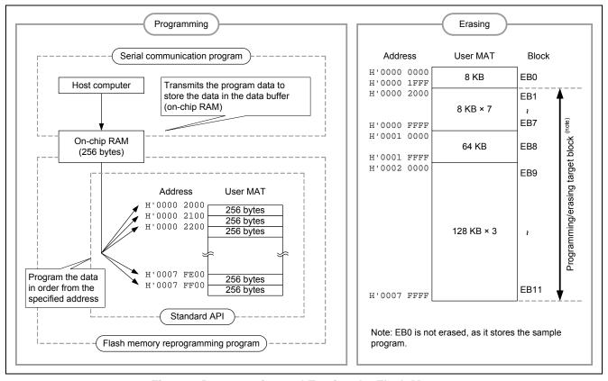
Figure 9 Programming and Erasing the Flash Memory
