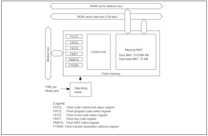
Figure 3 Flash Memory Block Diagram
