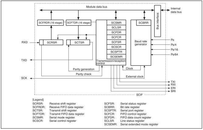
Figure 2 SCIF Block Diagram
