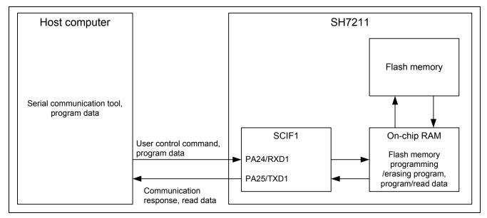
Figure 1 System Configuration
