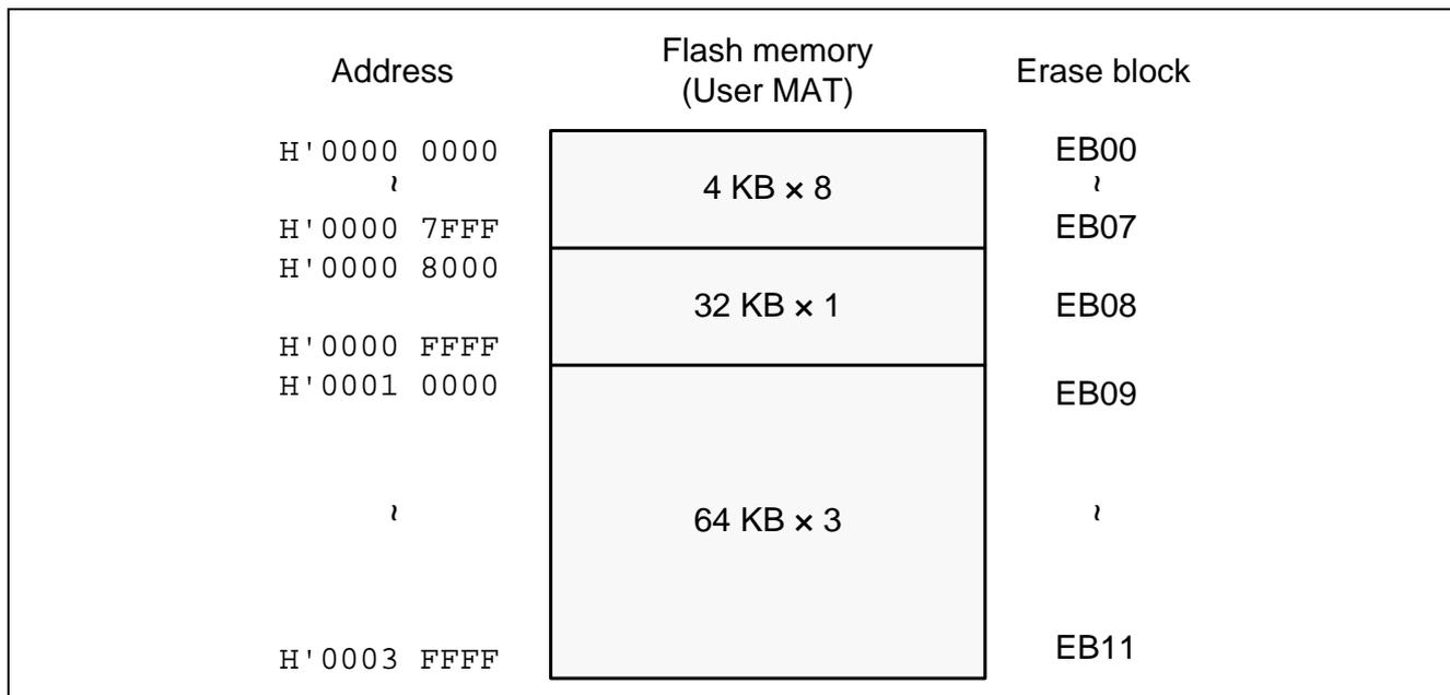
Figure 6 Dividing the Flash Memory Erase Block
