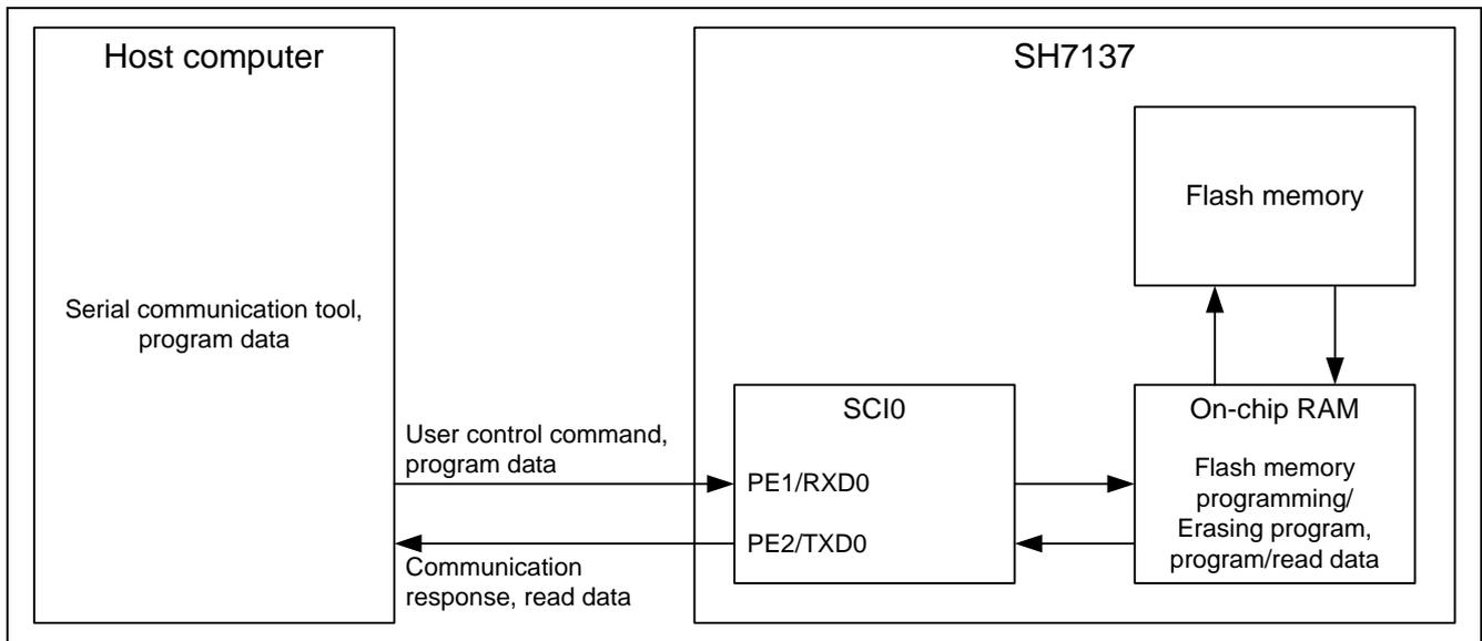
Figure 1 System Configuration
