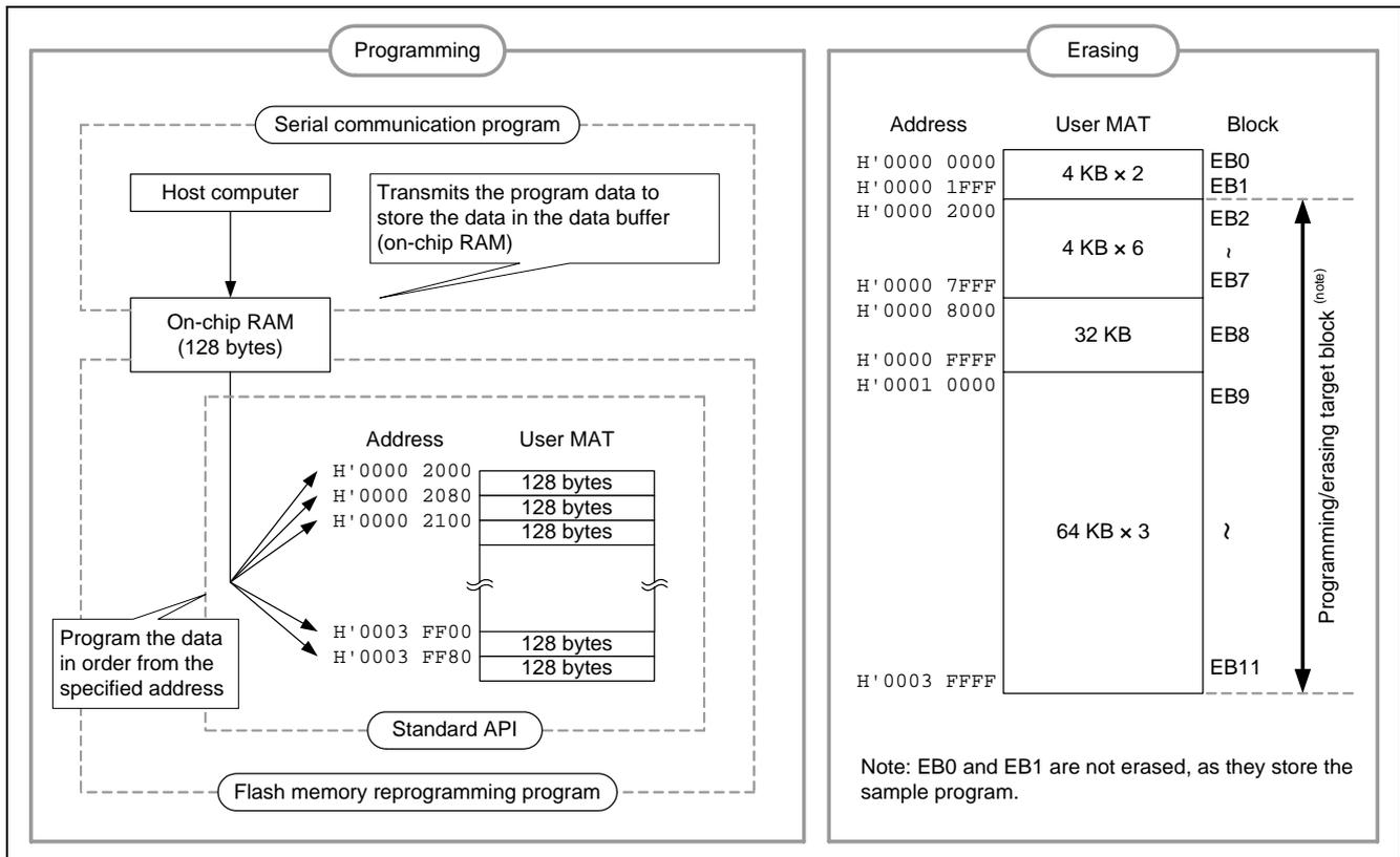
Figure 9 Programming and Erasing the Flash Memory
