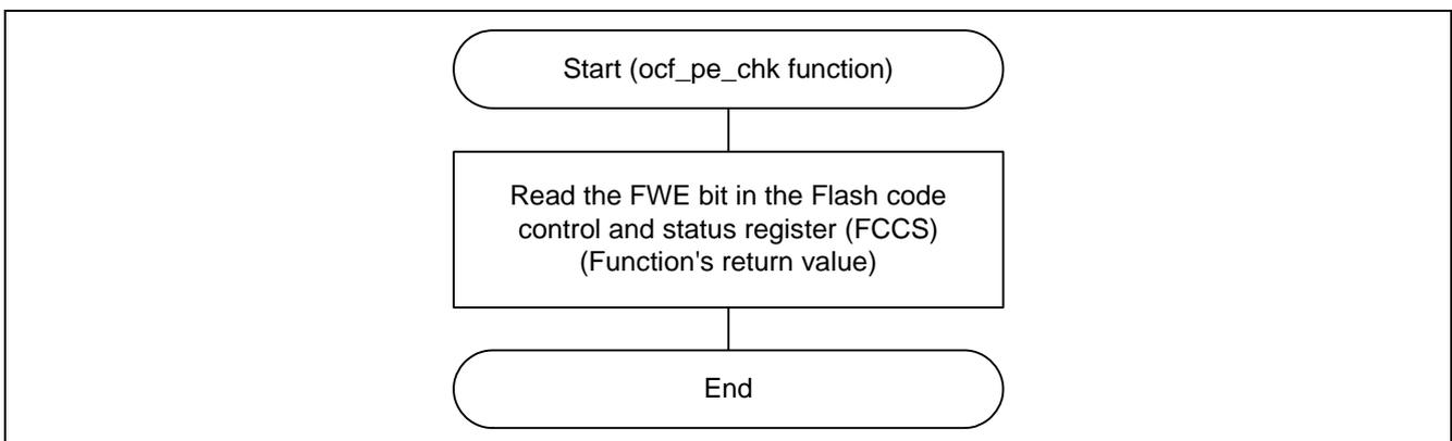
Figure 17 Checking the Flash Memory is Program-/Erase-enabled
