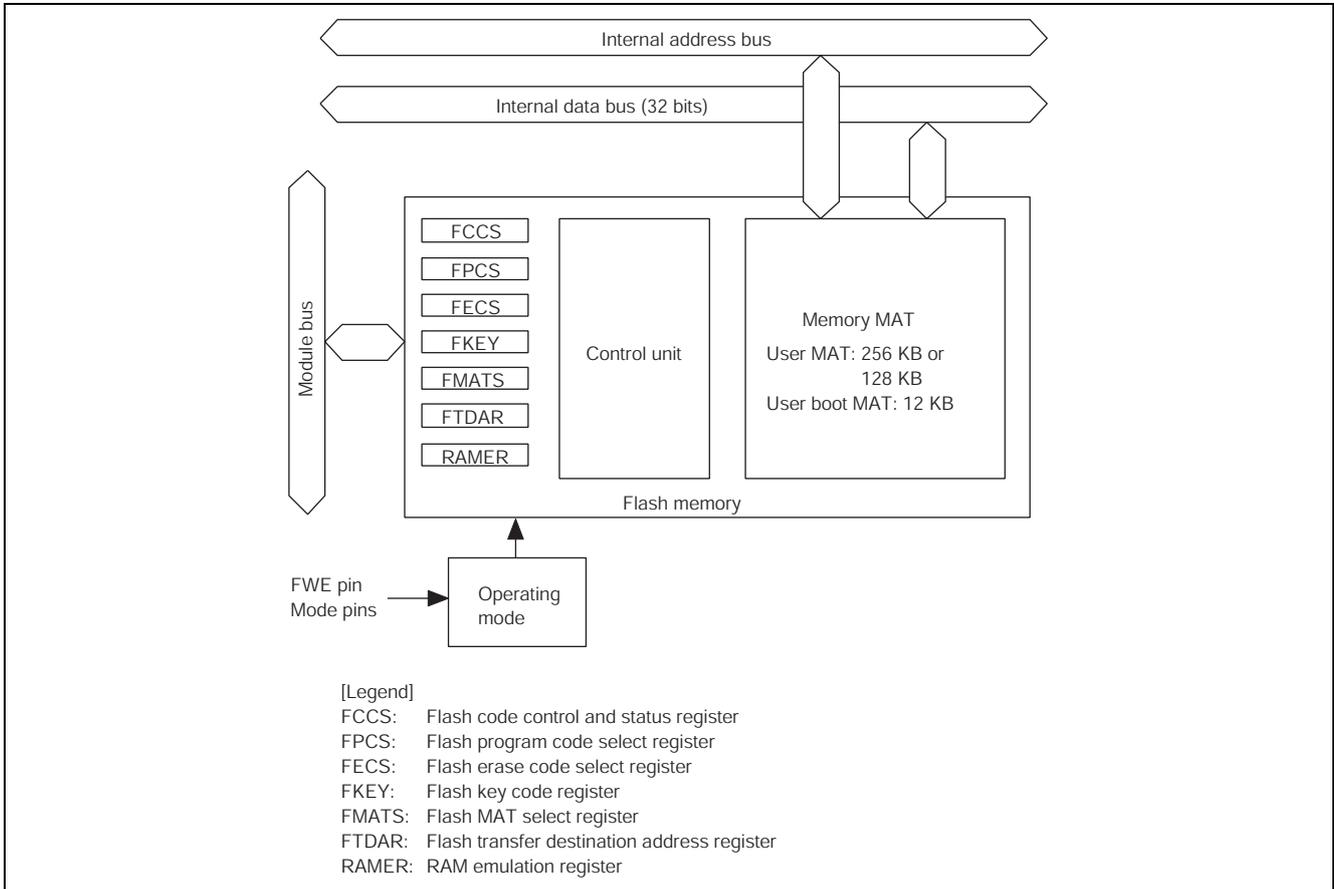
**Figure 3 Flash Memory Block Diagram**
