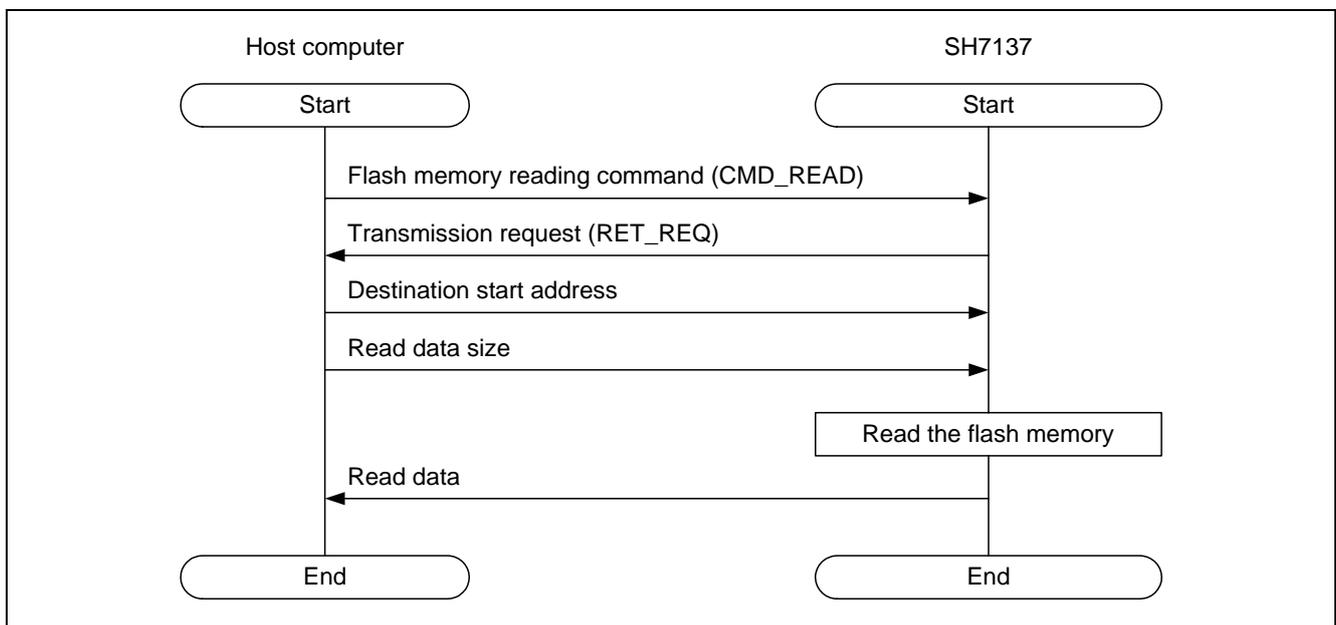
Figure 12 Communication Command Sequence When Reading the Flash Memory
