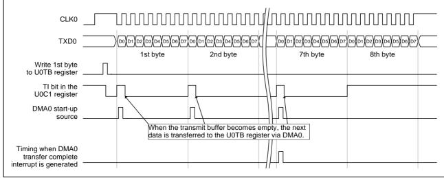
Figure 4.1 Continuous Transmit Timing Diagram
