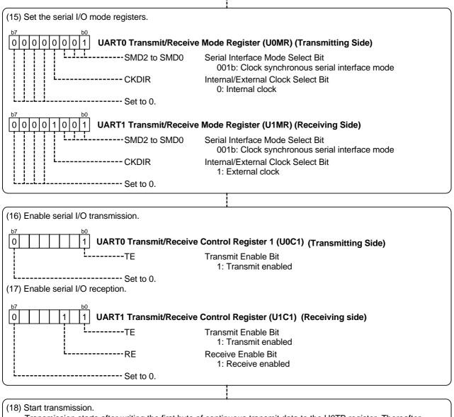
Transmission starts after writing the first byte of continuous transmit data to the U0TB register. Thereafter, data is continuously transmitted to the U0TB register via DMA0.
