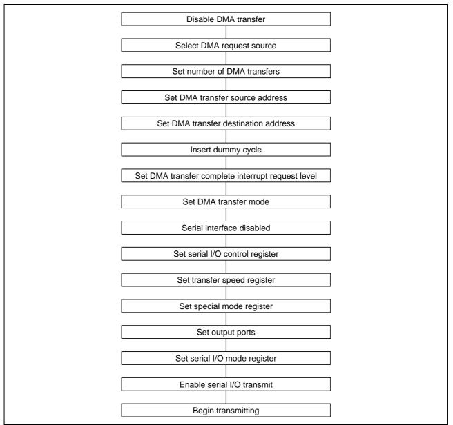
Figure 4.4 Serial Transmit Using DMAC
