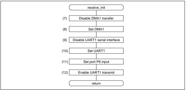
Figure 5.3 DMAC and UART Receive Initialization Function
