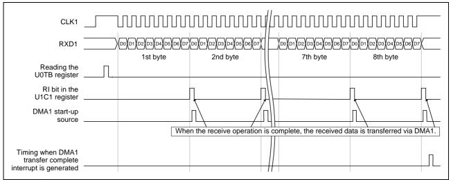
Figure 4.2 Continuous Receive Timing Diagram
