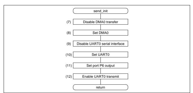
Figure 5.2 DMAC and UART Transmit Initialization Function
