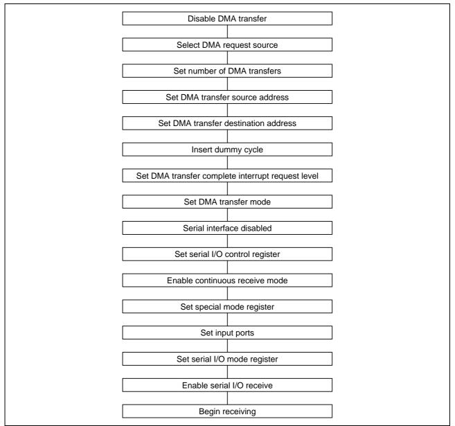
Figure 4.5 Receiving Side of Multi UART Transmit/Receive Using DMAC
