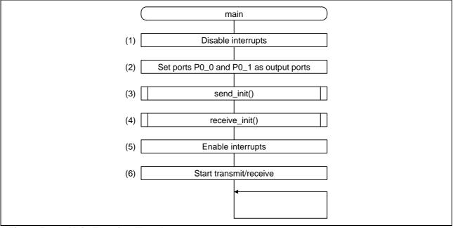
Figure 5.1 Main Function Flowchart
