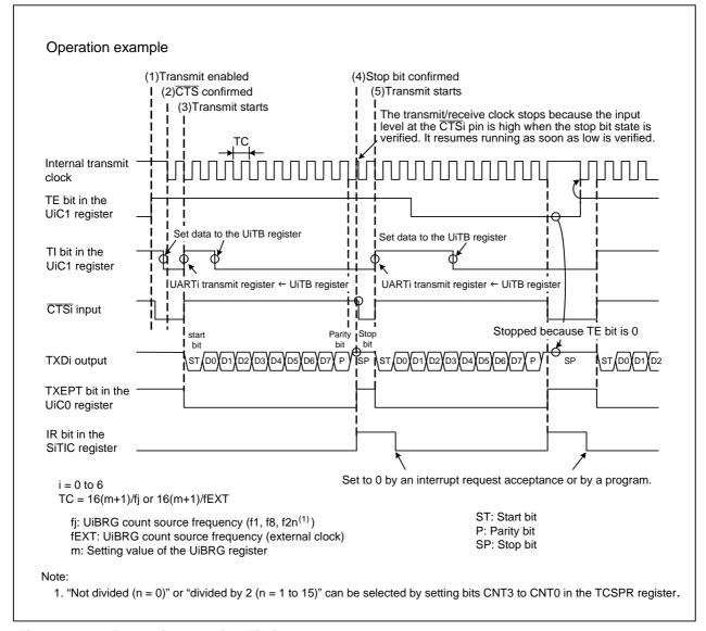
Figure 3.2 Transmit Operation Timing
