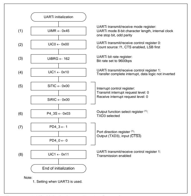
Figure 3.4 UARTi Initialization Process Flowchart (i = 0 to 6)
