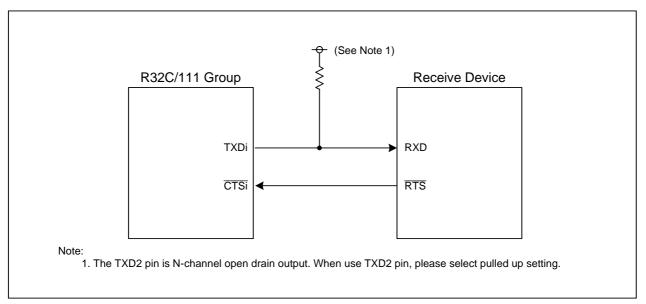
Figure 3.1 Connection Example for Transmission
