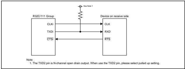
Figure 3.1 Connection Example for Transmission
