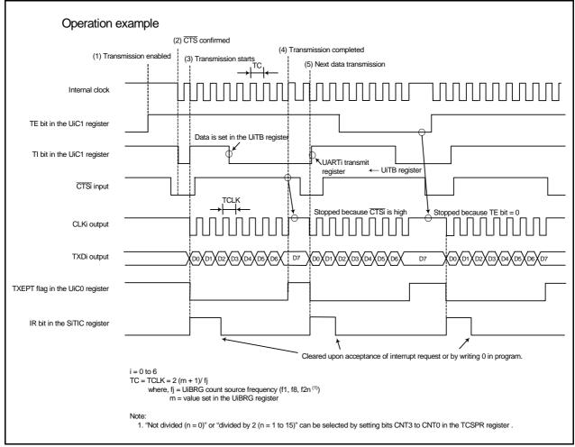
Figure 3.2 Transmit Operation Timing
