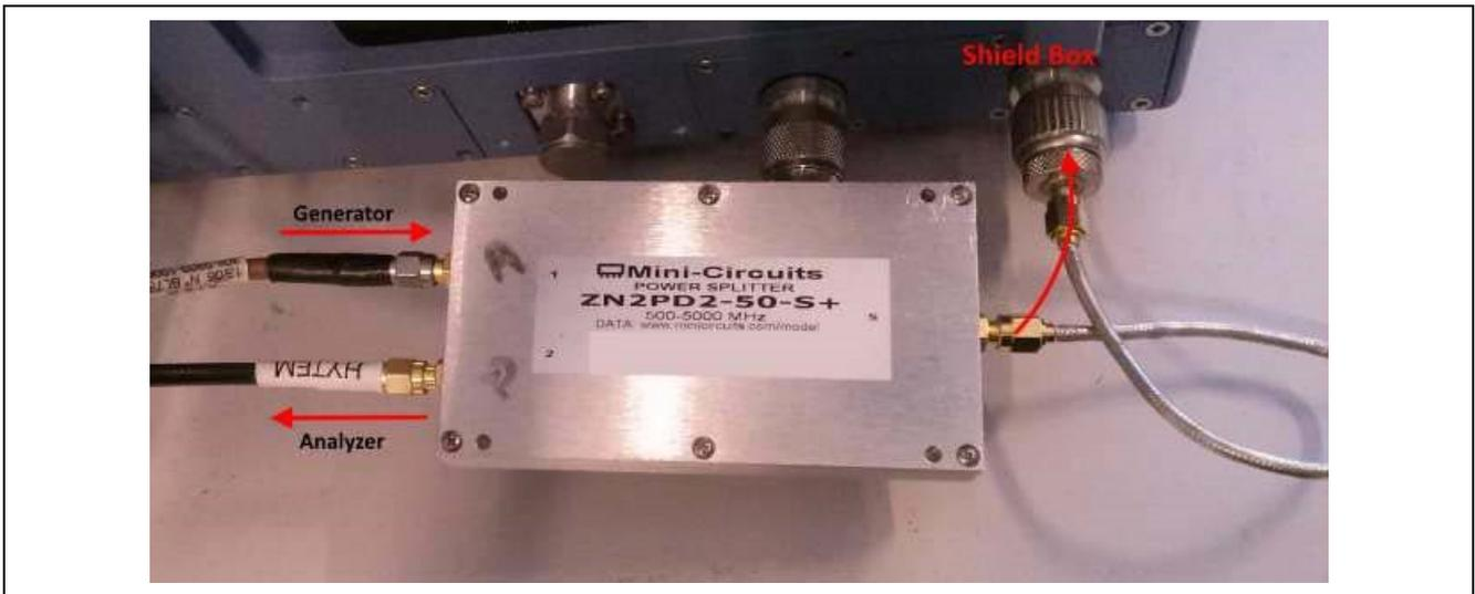
**Figure 26. Configuration for Calibration and Screening**
