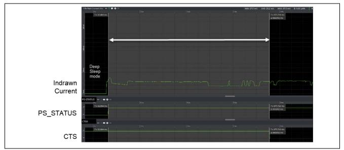
Figure 6. Modem Wakes Up from Deep Sleep Mode
