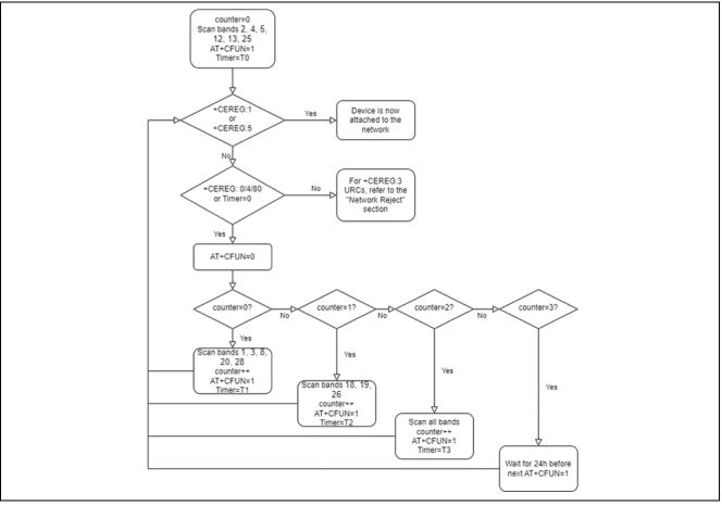
Figure 10. Out of Coverage Flowchart
