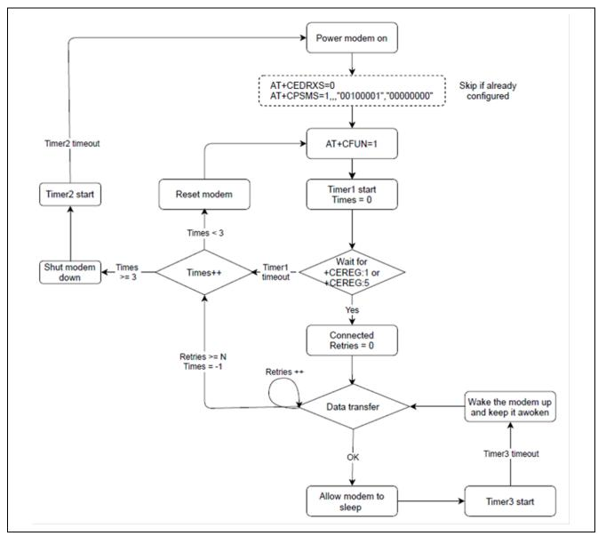
Figure 12. PSM Flow Example
