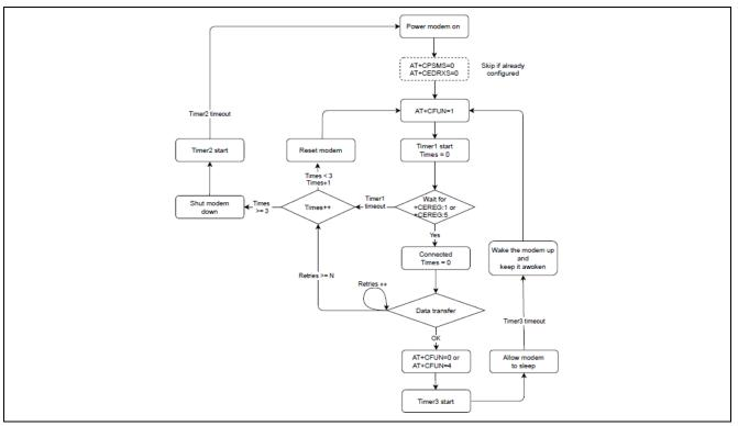
Figure 13. CFUN0/CFUN4 Use Case Example
