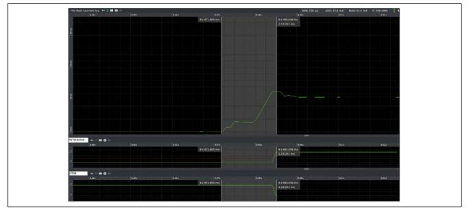
Figure 5. Modem Wakes Up from Sleep Mode
