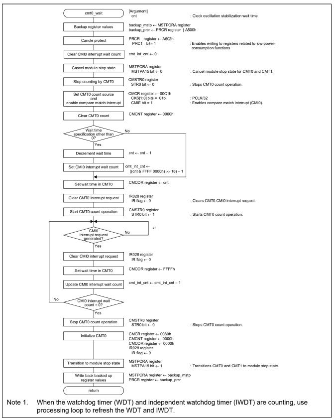
Figure 3.8 Software Wait Cycles Using CMT0
