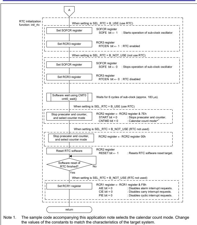
Figure 3.10 Sub-clock Oscillation Enable (2/2)
