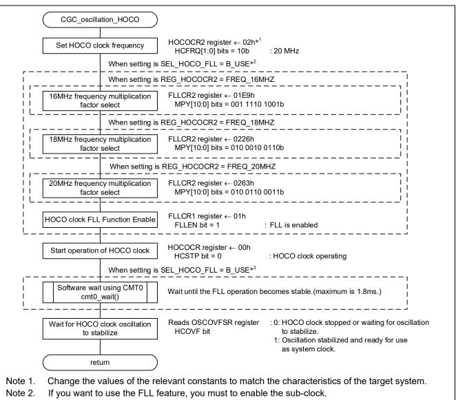
Figure 3.6 HOCO Clock Oscillation Enable
