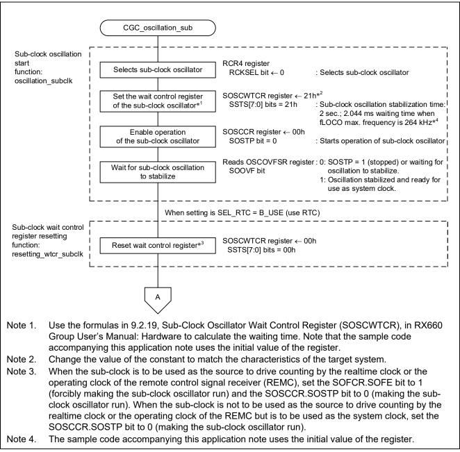
Figure 3.9 Sub-clock Oscillation Enable (1/2)
