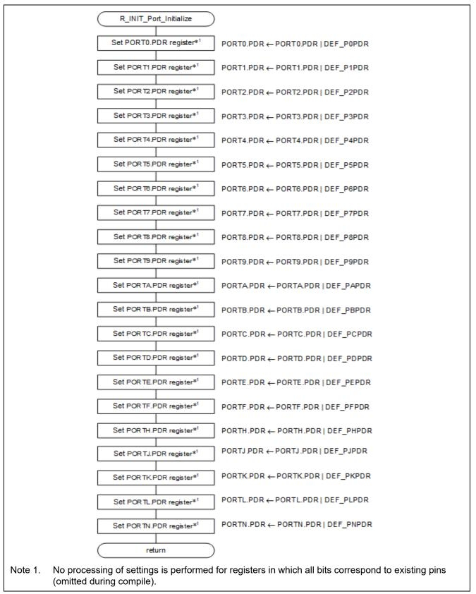
Figure 3.3 Initial Nonexistent Port Settings
