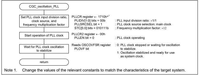
Figure 3.7 PLL Clock Oscillation Enable
