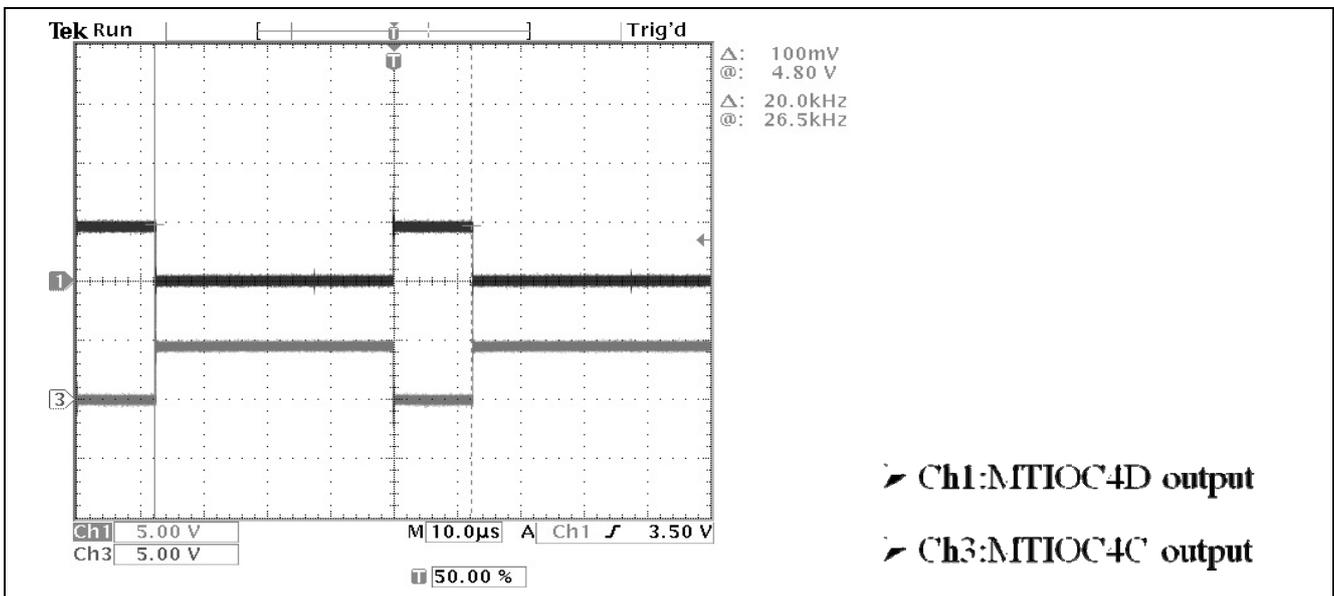
Figure 4-1 MTU3 output for 25% duty
