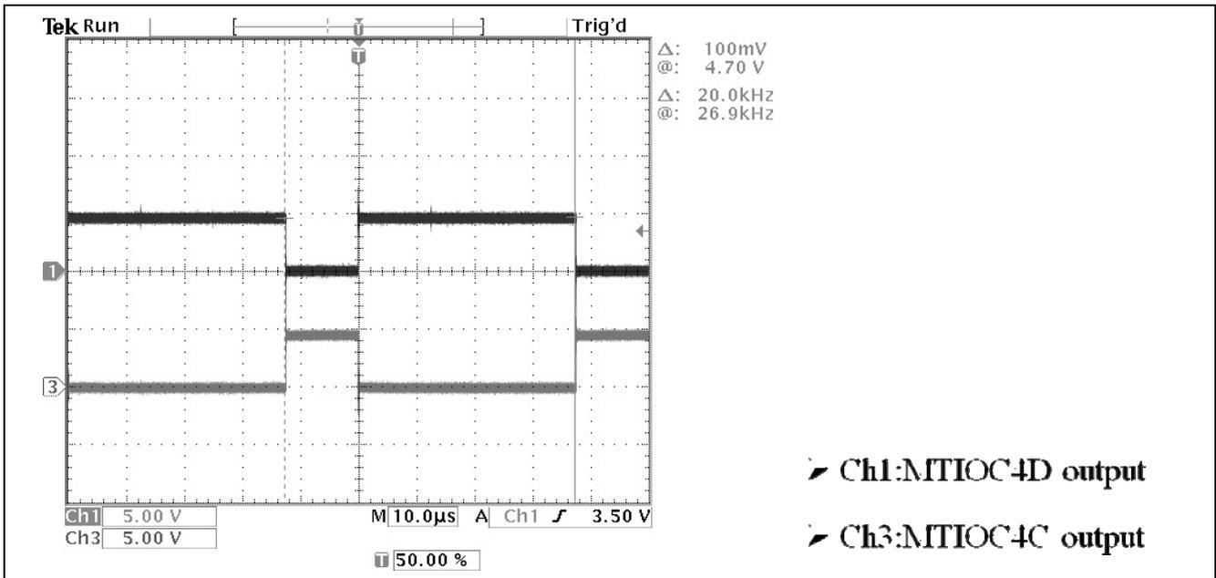
Figure 4-3 MTU3 output for 75% duty
