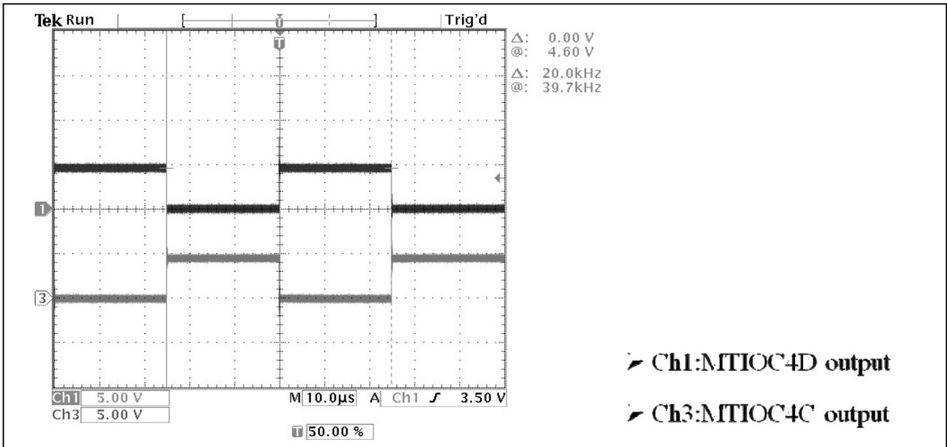
Figure 4-2 MTU3 output for 50% duty
