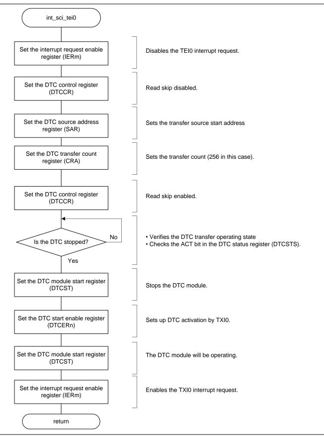
Figure 11 Transmit Complete Interrupt
