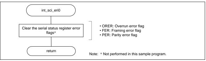
Figure 12 Receive Error Interrupt
