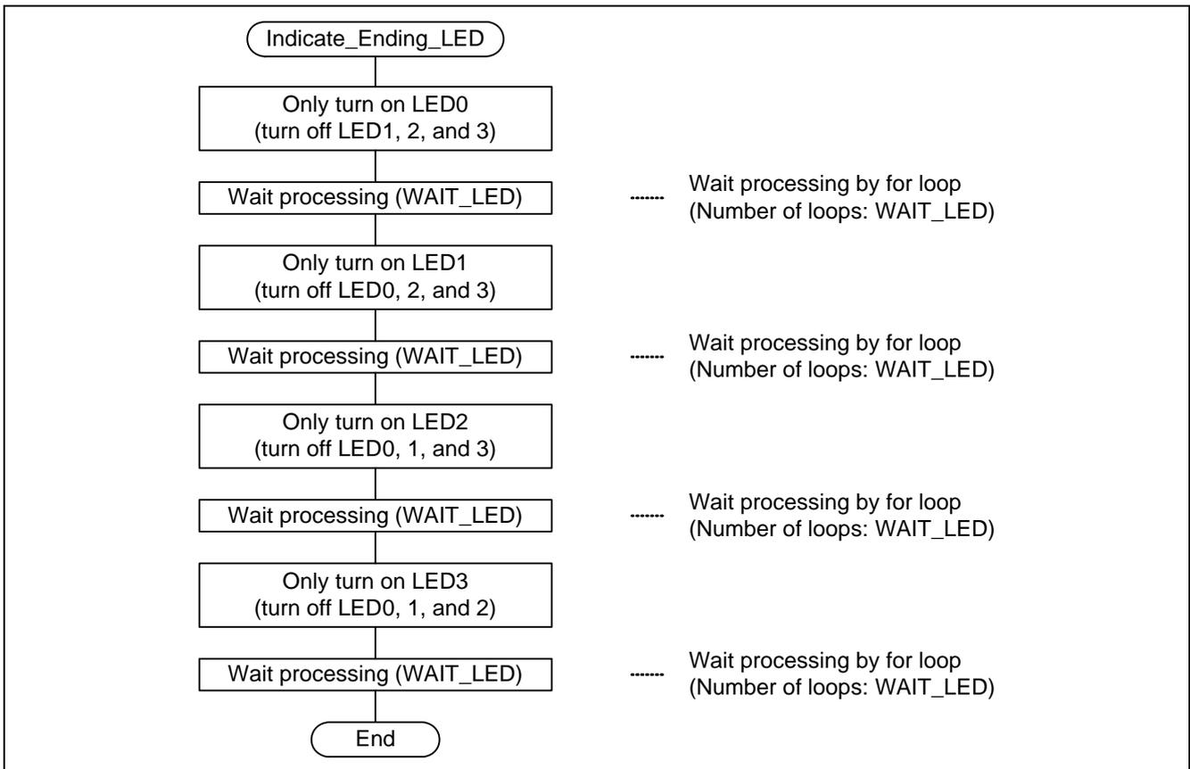
**Figure 16 Flowchart (Indicate\_Ending\_LED) (Master)**
