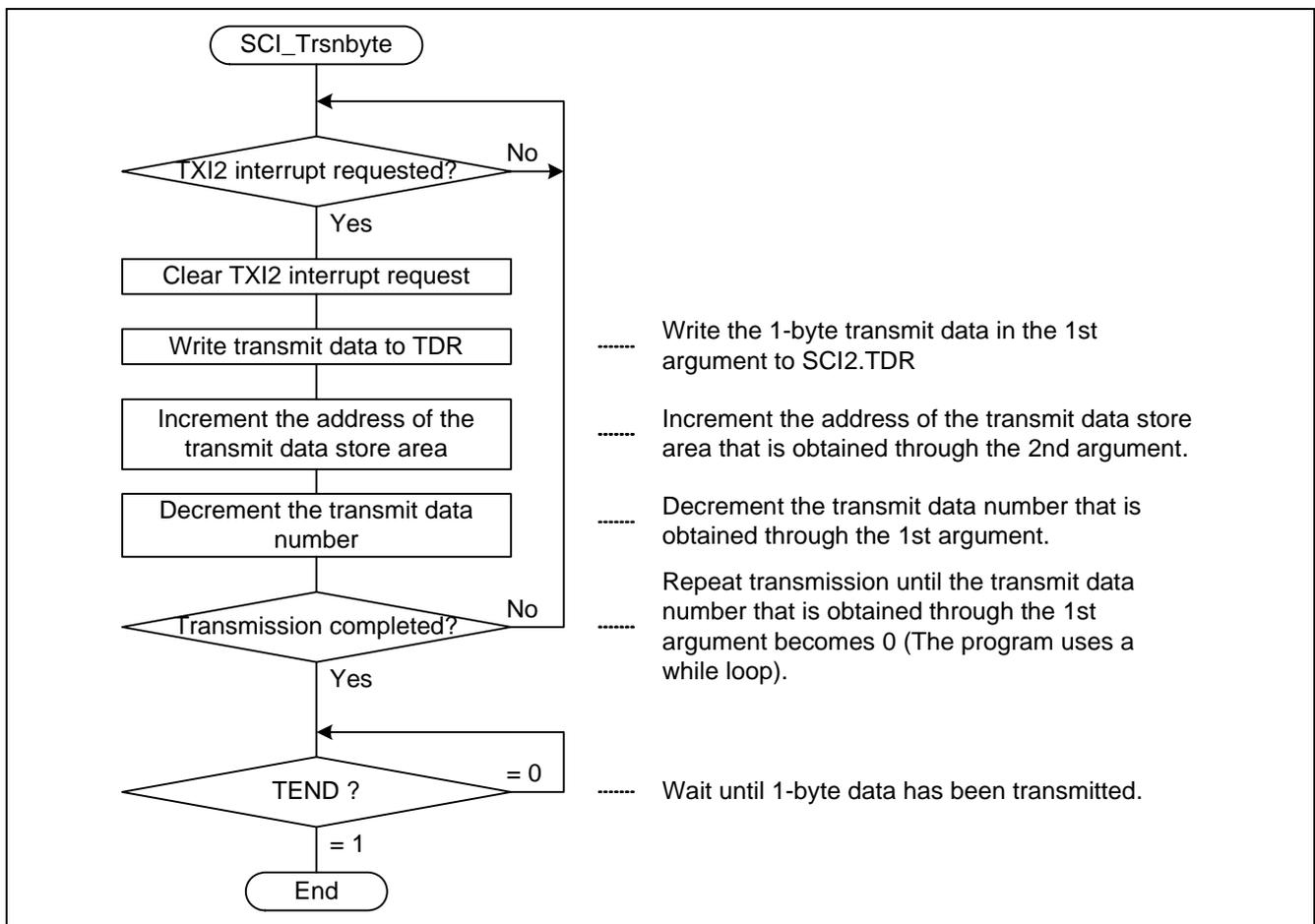
**Figure 18 Flowchart (SCI\_Trnsbyte) (Master)**
