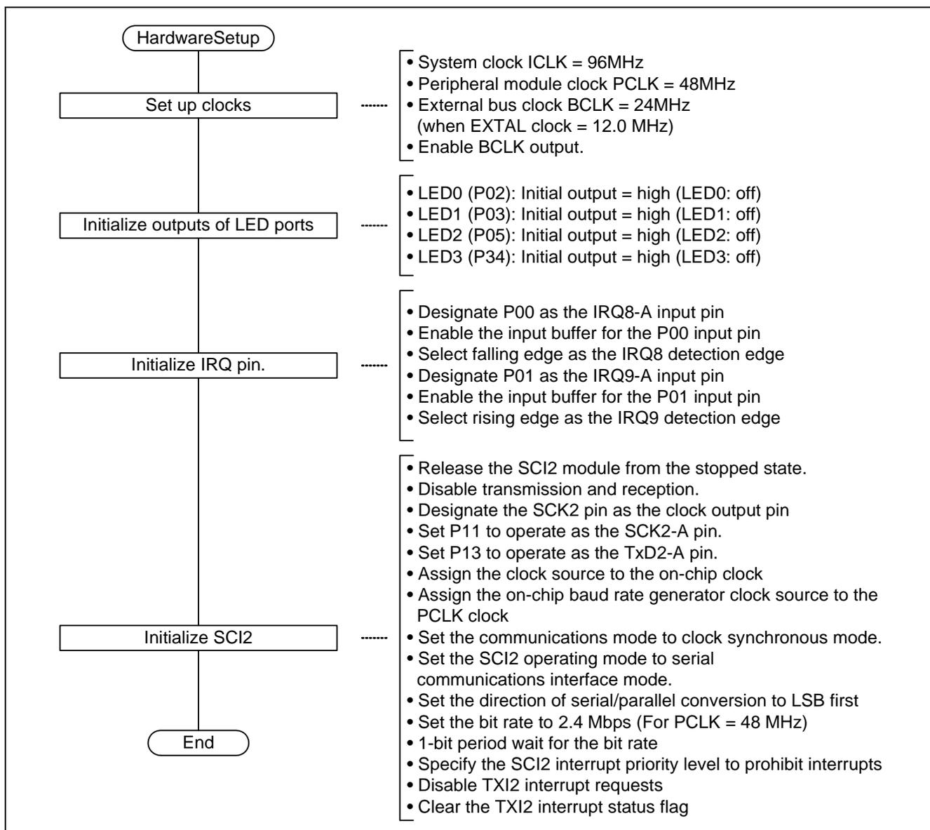
**Figure 13 Flowchart (HardwareSetup) (Master)**
