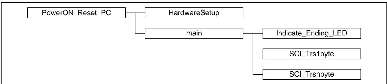
**Figure 11 Master Function Hierarchical Diagram**
