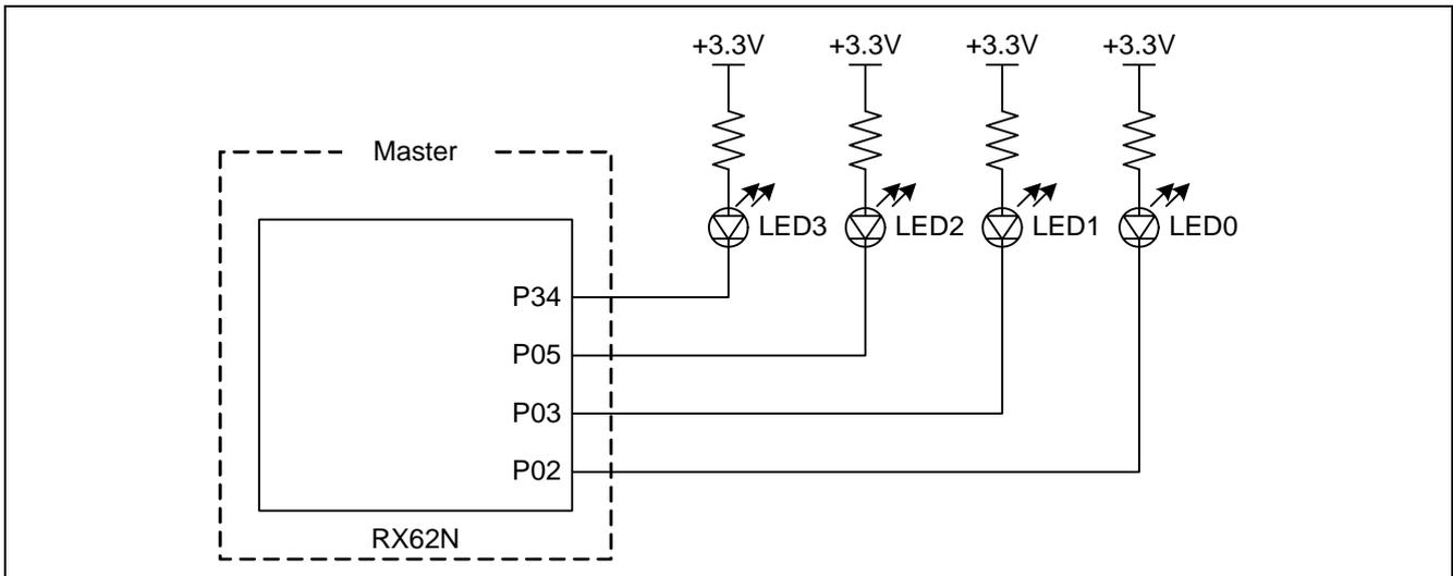
**Figure 9 Master LED Cabling Diagram**
