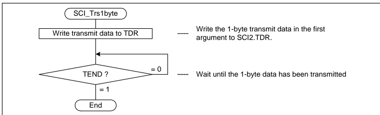
**Figure 17 Flowchart (SCI\_Trns1byte) (Master)**
