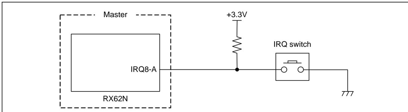
**Figure 10 Master IRQ Switch Connection Diagram**
