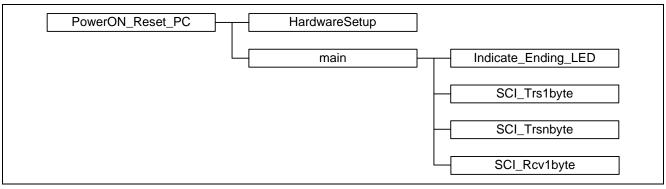
Figure 11 Master Function Hierarchical Diagram
