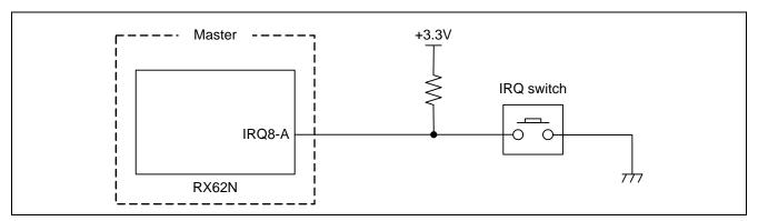
Figure 10 Master IRQ Switch Connection Diagram
