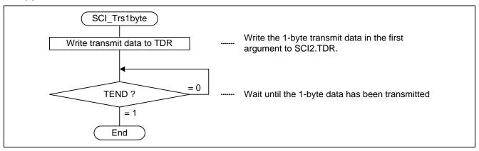
Figure 17 Flowchart (SCI\_Trs1byte) (Master)
