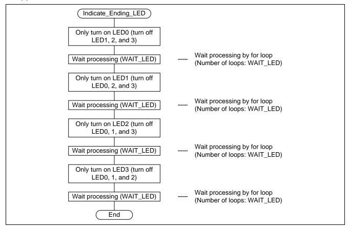
Figure 16 Flowchart (Indicate\_Ending\_LED) (Master)
