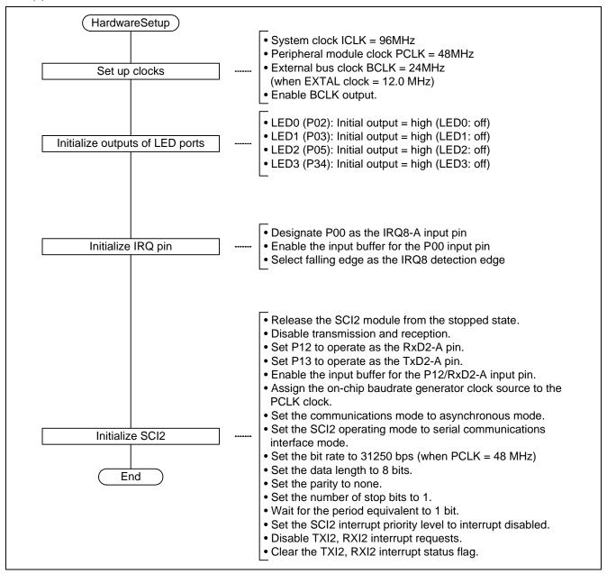
Figure 13 Flowchart (HardwareSetup) (Master)
