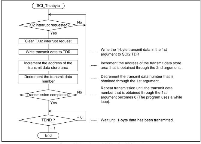
Figure 18 Flowchart (SCI\_Trsnbyte) (Master)
