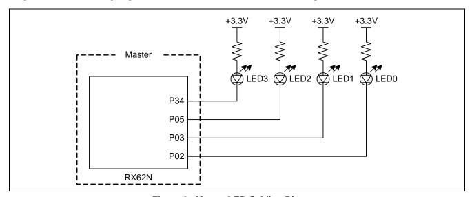
Figure 9 Master LED Cabling Diagram
