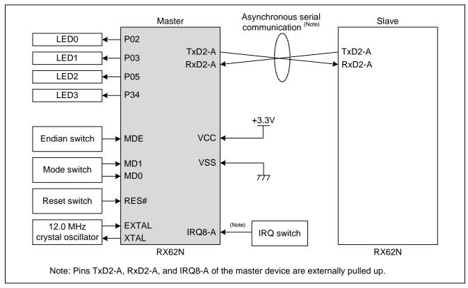
Figure 2 Master Hardware Configuration Diagram
