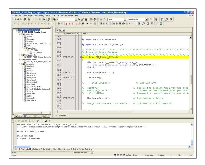
Press short-cut key "F5" to allow the program to run. Optionally, Debug → Go may be selected as shown:
