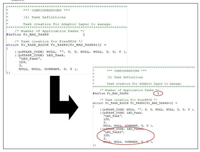
Note that fr\_MAX\_TASKS has been updated to 2 and an initialization of LED\_Task2 has been created. This task structure initialization is necessary for the Adaptor Layer to manage the Tasks. For more information, consult the Adaptor Layer User Manual and API Specification Application Note.
