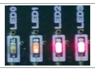
This time, LED0 blinks with a delay of 200ms while LED1 through LED3 blinks with a delay of 500ms.
