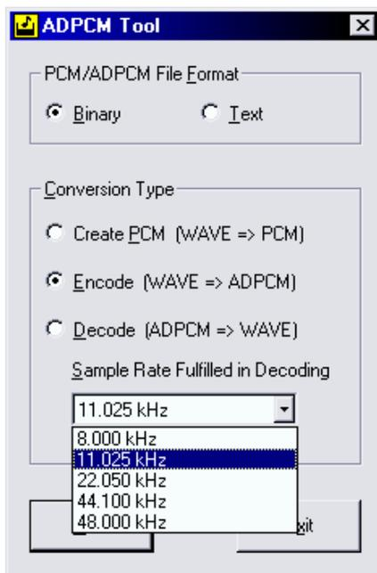
**Figure 10.** The ADPCM Tool is a GUI for converting back and forth between ADPCM and WAV formats. After selecting what format types to convert between and sampling frequency, press 'Go' to select the file to convert.
