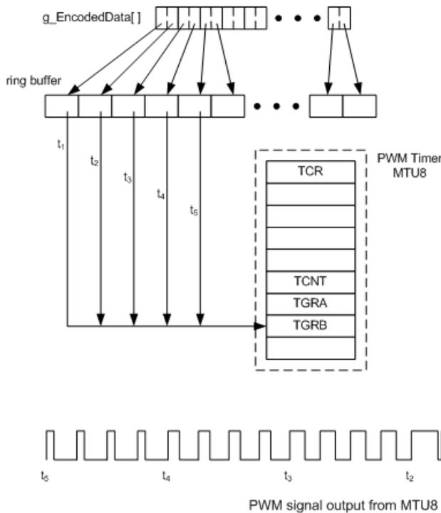
The application decompresses a segment of the ADPCM file into the ring buffer and starts the DTC transfer. While the transfer occurs, the application decodes another segment of the file. When the DTC completes, it interrupts the CPU, the DTC is set up to transfer the next segment and then started.
