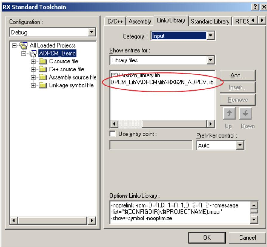
Figure 8 In the “Category” pull down, select “Input” and then “Library files” in the “Show entries for” pull down. Double click on the entry circled in red above.
