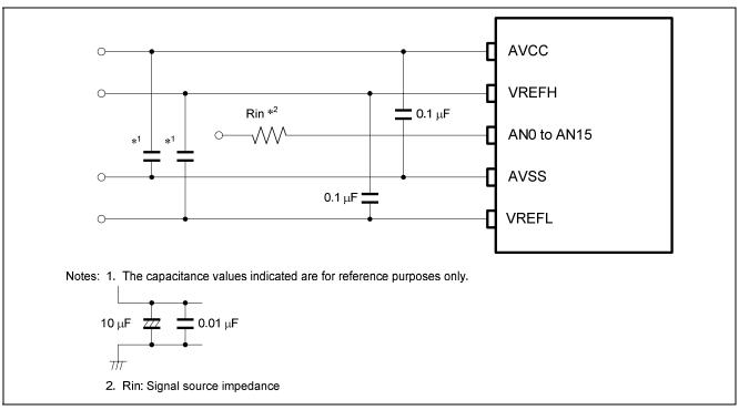
Figure 3 Reducing Noise in Power Supply Lines
