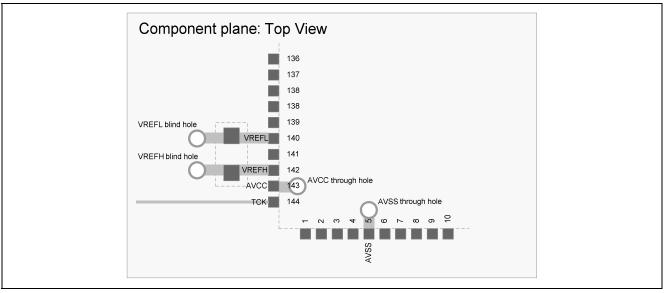
Figure 4 RX610 LQFP Package TCK and AVCC Pins
