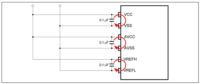
Figure 1 Power Supply Pin Capacitors and Closed Loops
