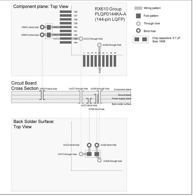
Figure 2 RX610 LQFP Package Power Supply Pin Capacitor Layout Example
