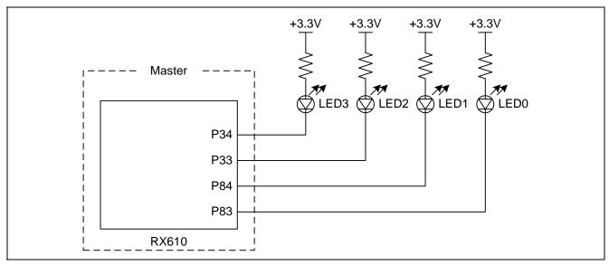
Figure 9 Master Device LED Connection Diagram
