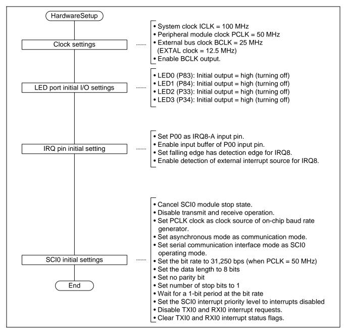
Figure 13 Flowchart (HardwareSetup) (Master)
