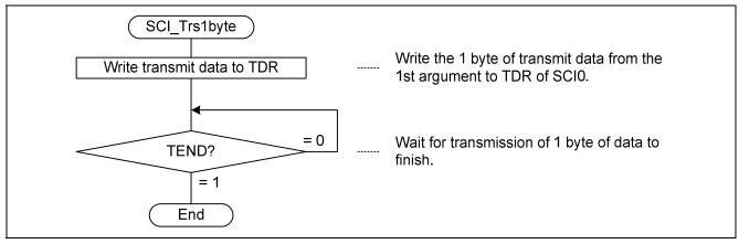
Figure 17 Flowchart (SCI\_Trs1byte) (Master)
