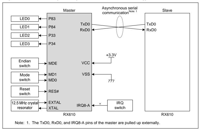
Figure 2 Hardware Configuration Diagram of Master Device
