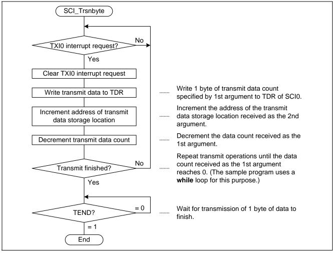
Figure 18 Flowchart (SCI\_Trsnbyte) (Master)
