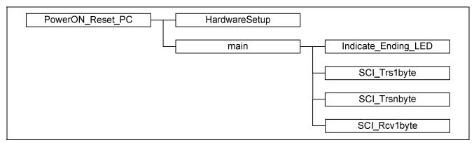
Figure 11 Hierarchy of Master Device Functions
