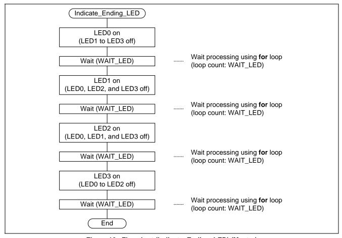
Figure 16 Flowchart (Indicate\_Ending\_LED) (Master)
