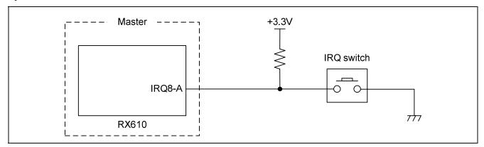
Figure 10 Master IRQ Switch Connection Diagram
