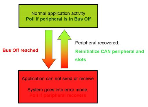
Figure 5. Handling recovery from Bus Off for the application. (The MCU detects recovery of the bus on its own.)
