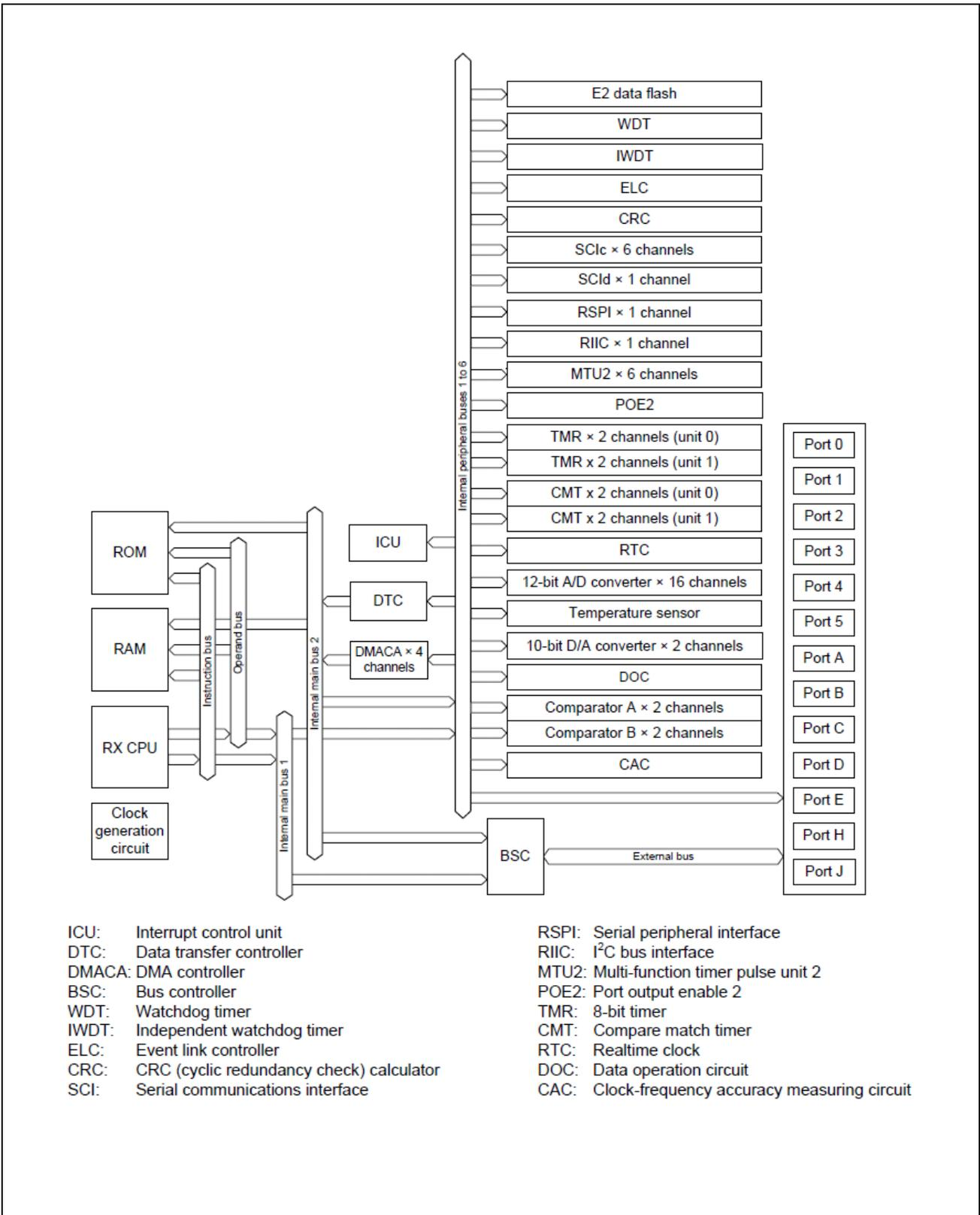
Figure 3 Block Diagram of RX210
