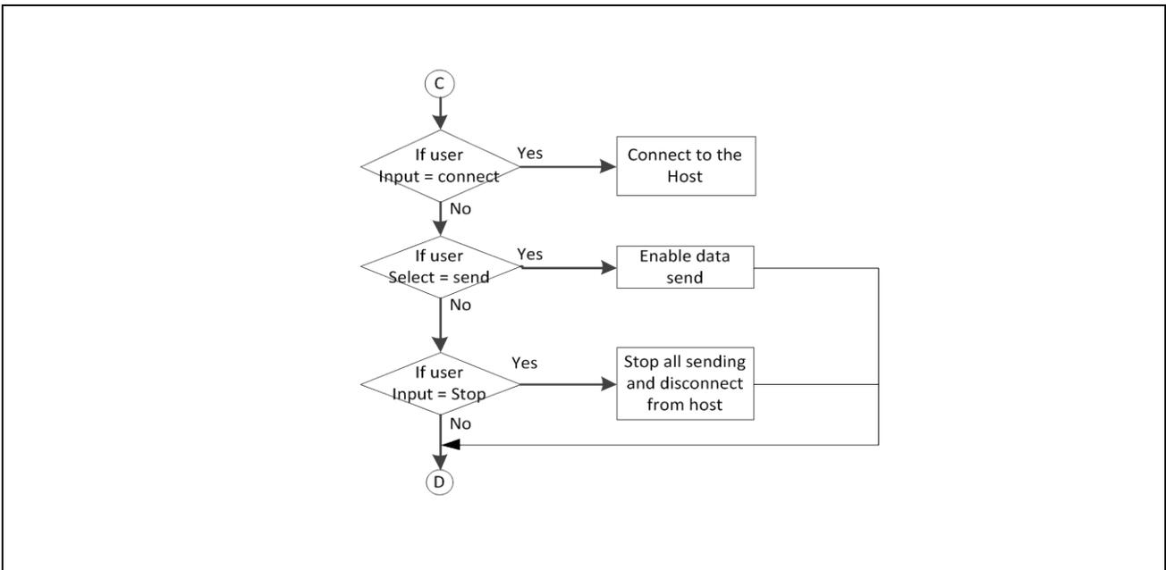
Figure 9 Communication Software Flow Chart
