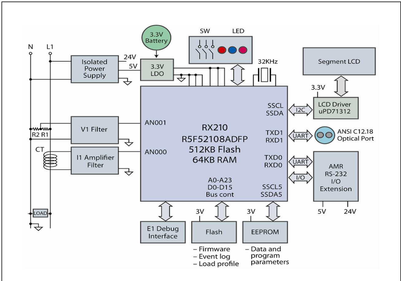
Figure 4 Reference Design of Energy Meter using RX210
