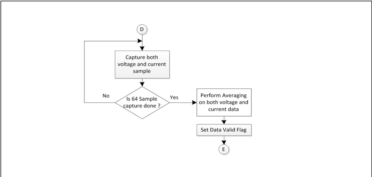
Figure 10 Front end signal Processing Flow chart
