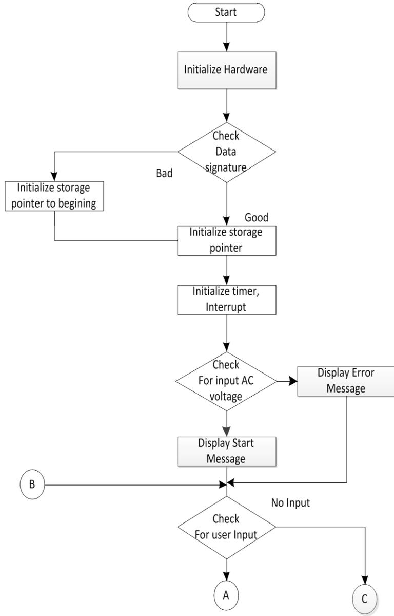
Figure 7 Meter Initialization flow chart
