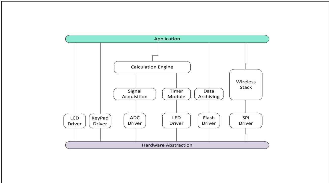
Figure 6 Software Architecture of Energy Meter
