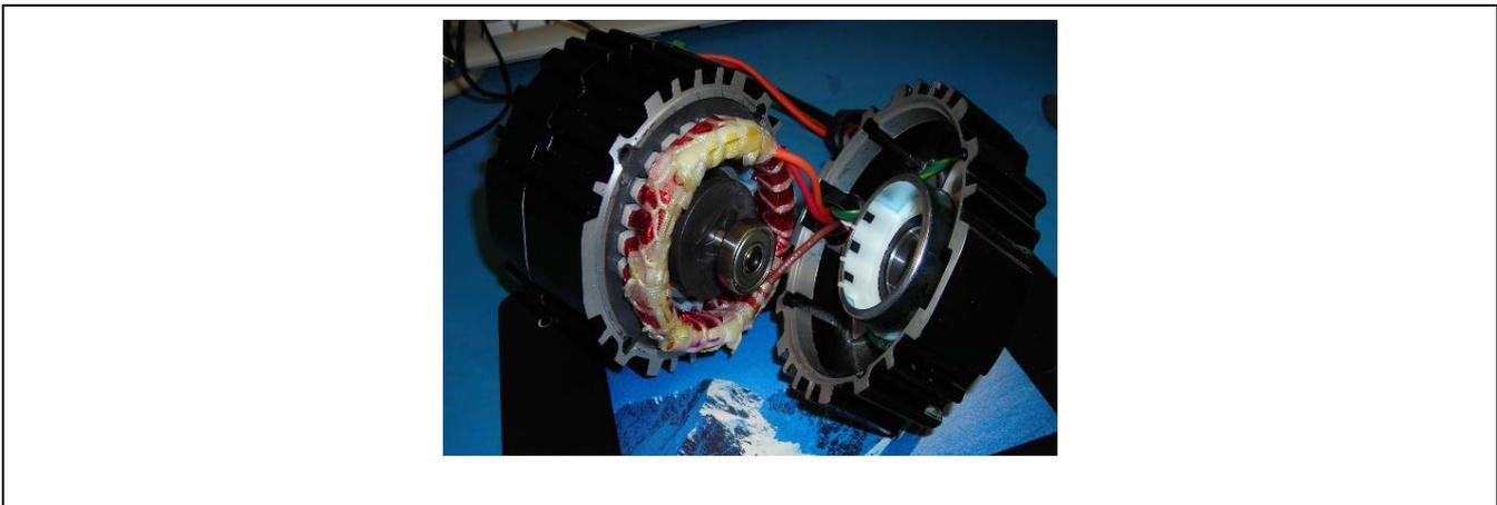
**Figure 13 A physical BLDC motor for parameter tuning**
