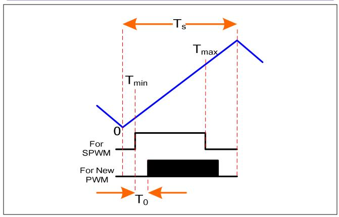
Figure 7 Diagram of  $T_0$  component calculation
