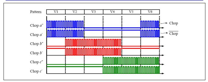
Figure 15 Three phase conduction mode
