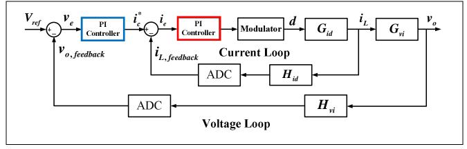
Figure 3 Block diagram of the developed PFC
