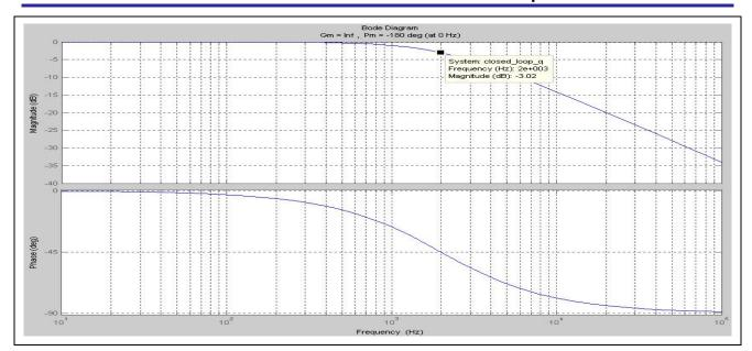
Figure 11 Bode plot of q-axis current controller
