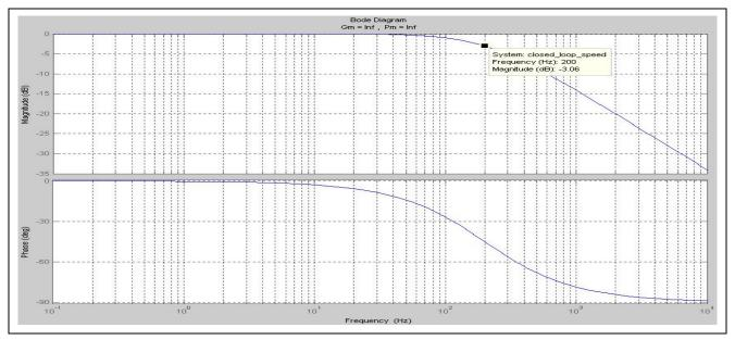
Figure 13 Bode plot of speed controller
