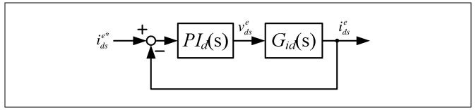
Figure 8 Block diagram for d-axis current controller design
