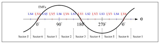
Figure 16 The relationship of rotor position
