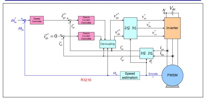
Figure 6 Block diagram of vector-controlled PMSM drives
