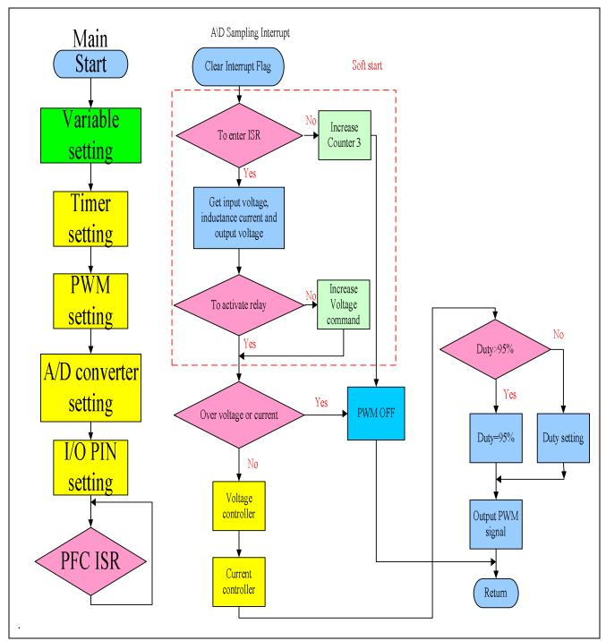
Figure 17 Flow chart of PFC software implementation
