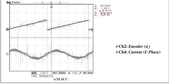
Figure 26 Relationship between encoder signal and U phase current
