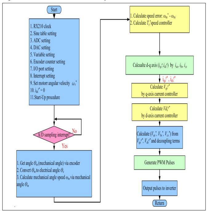
Figure 18 Flow chart of motor control software implementation
