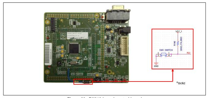
Figure 20 RX210-based control board
