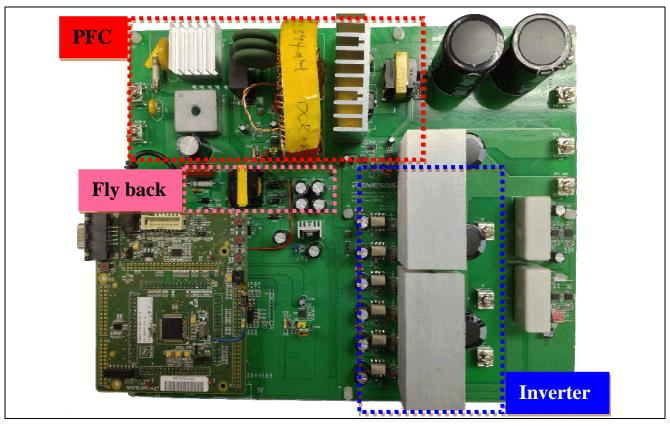
Figure 19 Experimental set up
