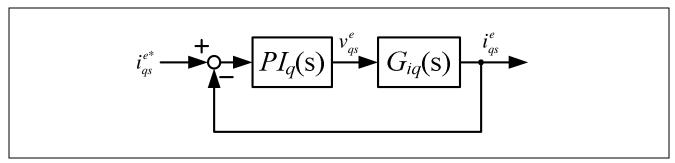
Figure 10 Block diagram for q-axis current controller design
