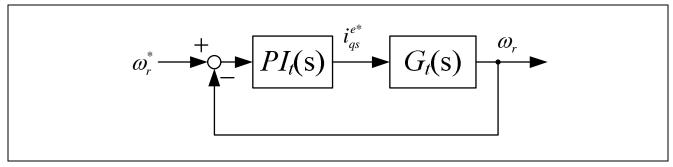
Figure 12 Block diagram for speed controller design
