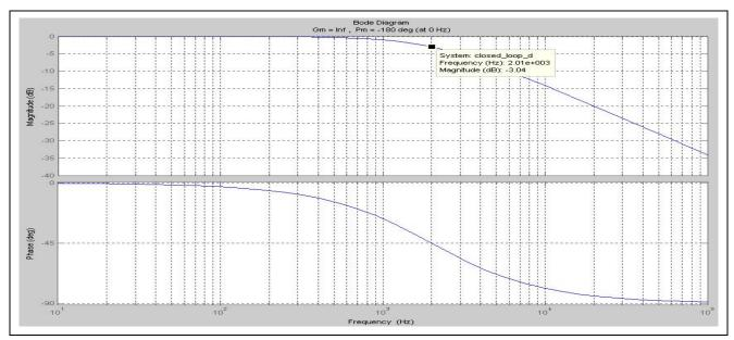
Figure 9 Bode plot of d-axis current controller
