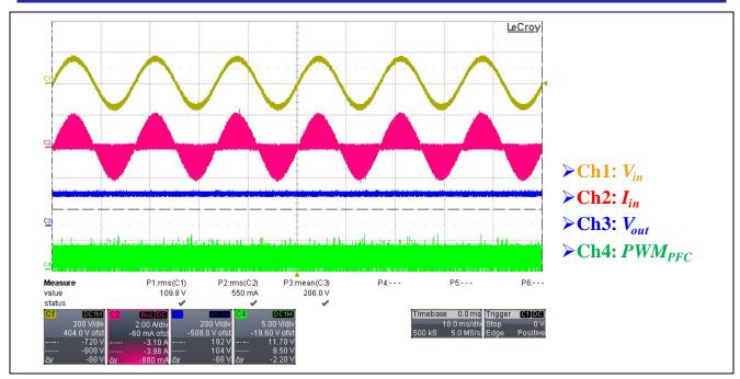
Figure 25 Measured waveforms of motor control with PFC
