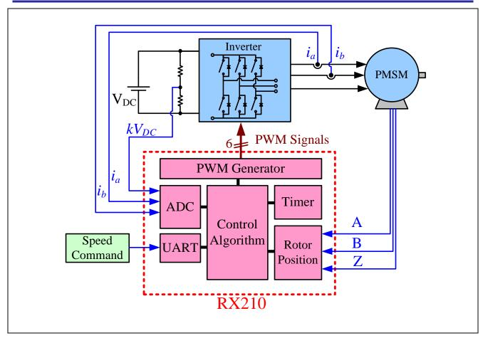
Figure 2 Vector-controlled PMSM drive
