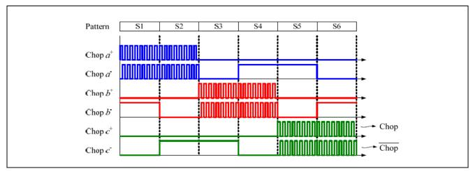
Figure 14 Two phase conduction mode
