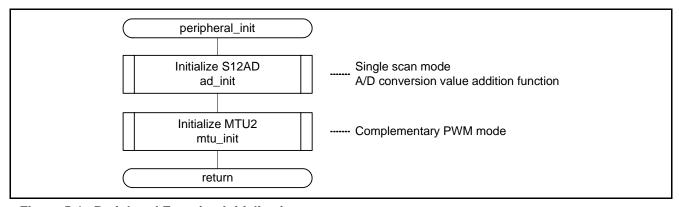
Figure 5.4 Peripheral Function Initialization
