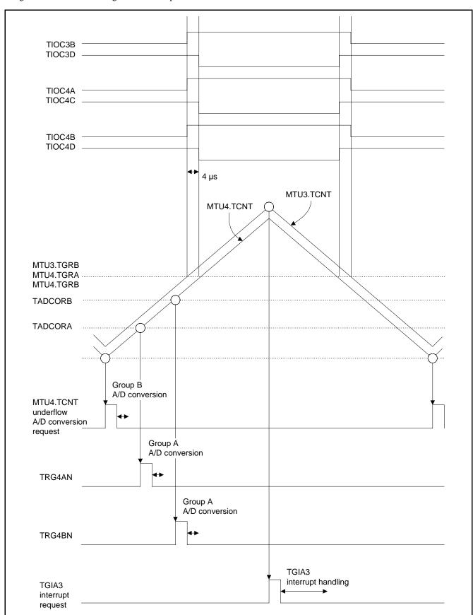
Figure 5.1 shows the timing for MTU2a operation and A/D conversion.
