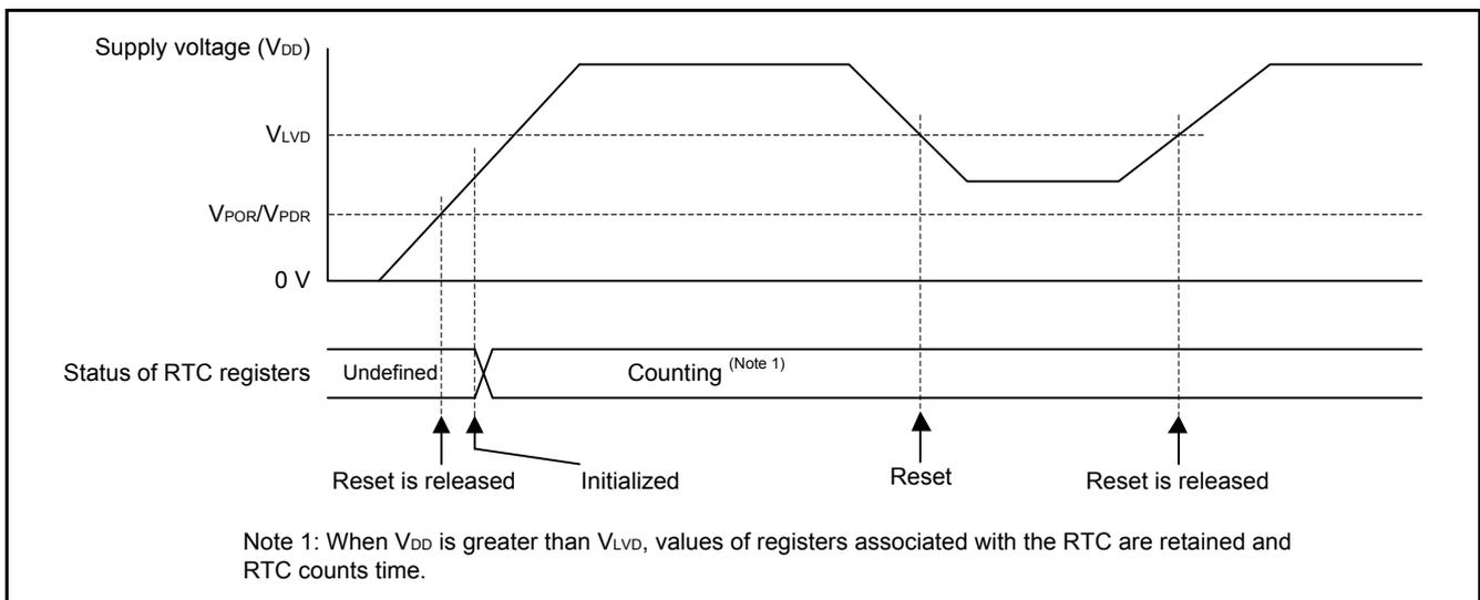
**Figure 1.1 Operation Overview of Supply Voltage Shift and Data Retention**
