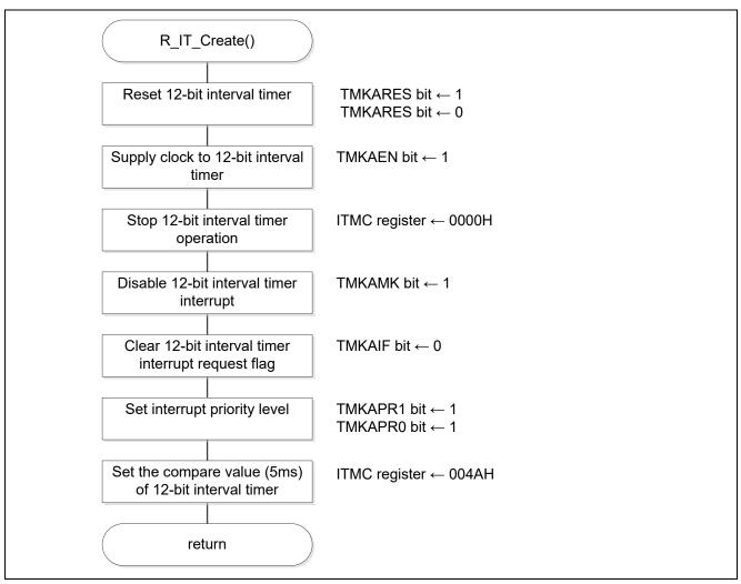
Figure 5.7 12-bit Interval Timer Setting
