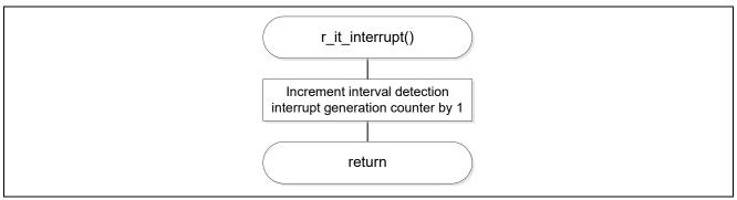
Figure 5.76 12-bit Interval Timer Interrupt Servicing
