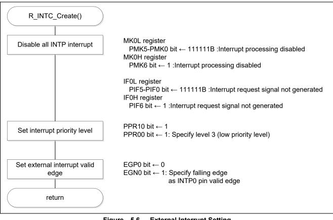
Figure 5.6 External Interrupt Setting
