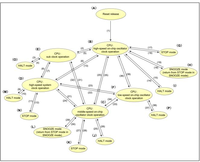
Figure 1.1 Operating Mode Status Transition Diagram
