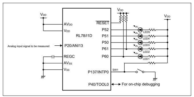
Figure 4.1 Hardware Configuration
