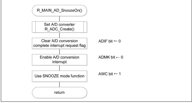
Figure 5.39 A/D Converter Setting
