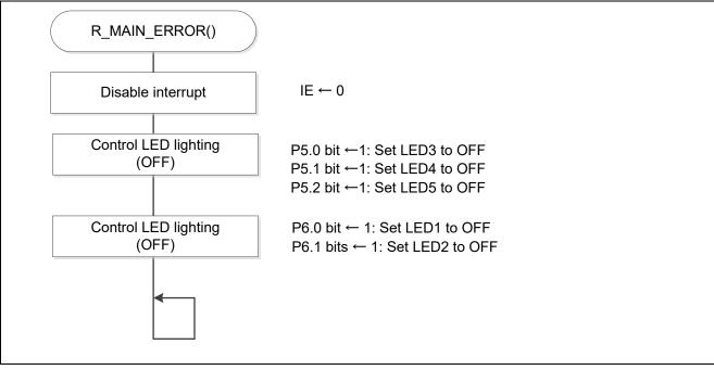
Figure 5.17 Error Processing of Status Transition
