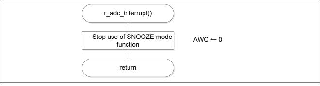
Figure 5.77 A/D Conversion Completion Interrupt Servicing
