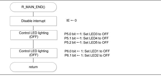
Figure 5.74 Status Transition End Processing
