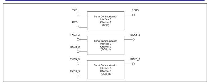
Figure 1.1 Block diagram of the serial communication interface 3 (SCI3)
