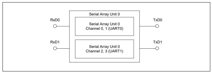
Figure 1.2 Block Diagram of Serial Array Unit 0 (SAU0) UART
