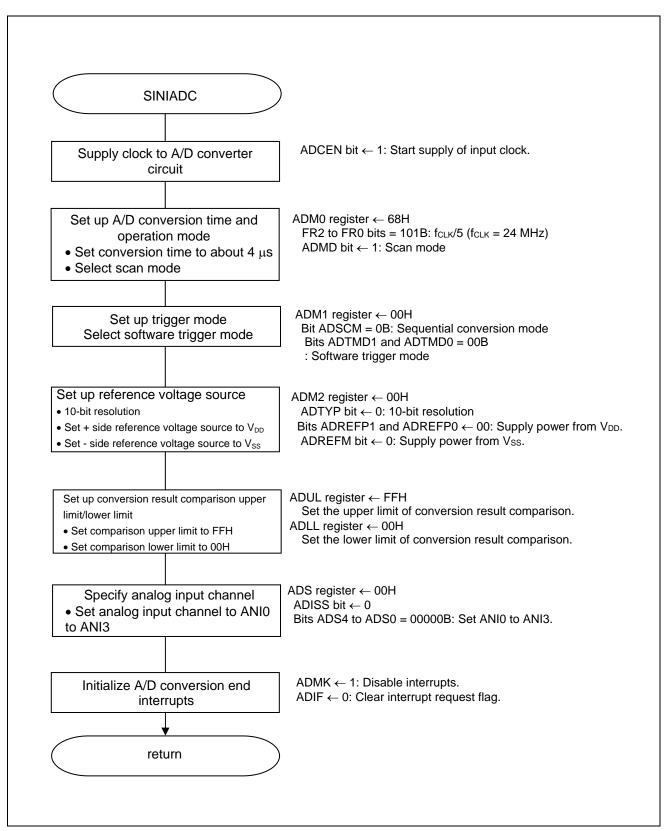
Figure 5.6 Initial Setup of A/D Converter
