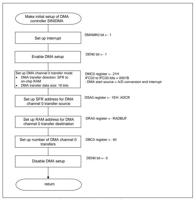
Figure 5.5 Initial Setup of DMA Controller
