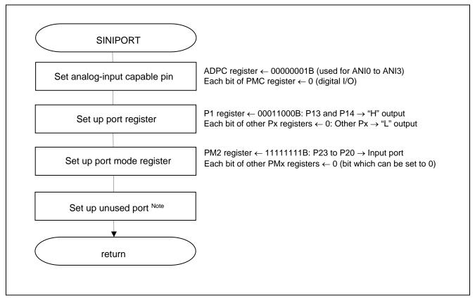
Figure 5.3 I/O Port Setup Function
