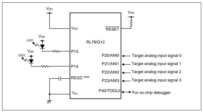
Figure 4.1 **Hardware Configuration**
