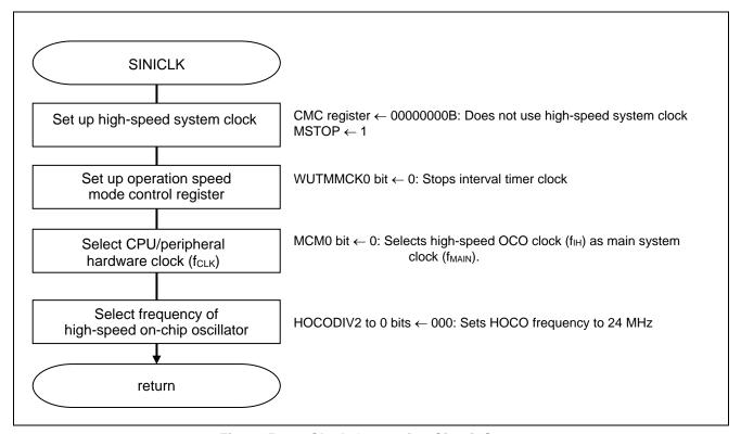
Figure 5.4 Clock Generation Circuit Setup
