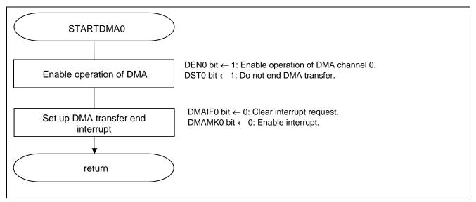
Figure 5.7 Enabling the DMA Controller
