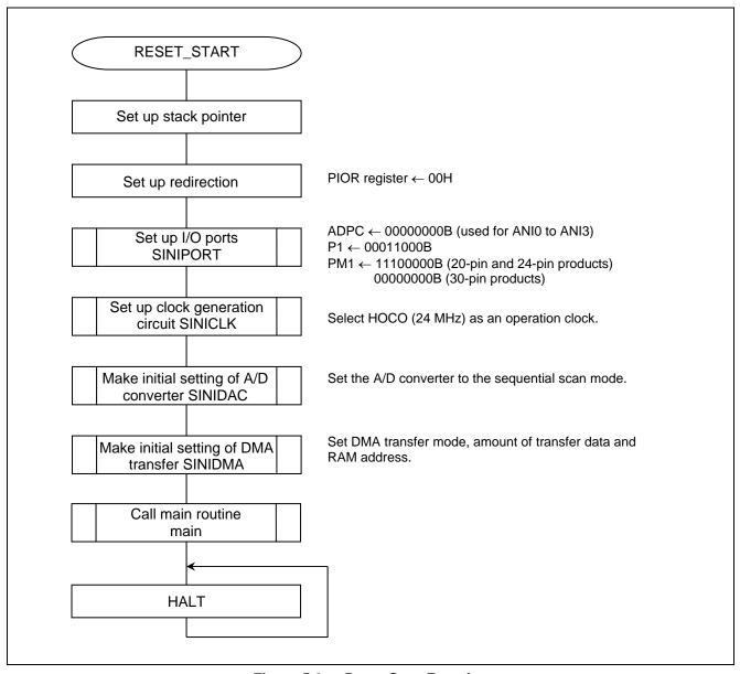
Figure 5.2 Reset Start Function
