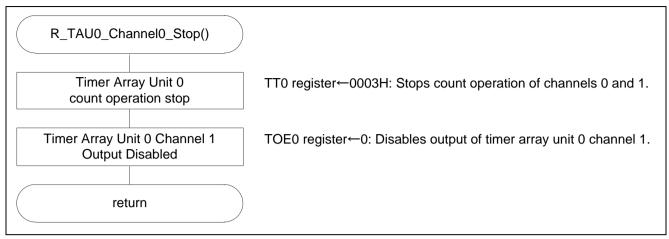
Figure 5.17 Stopping Timer Array Unit 0 Operation
