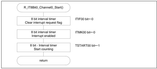
Figure 5.8 Starting 8-Bit Interval Timer Operation
