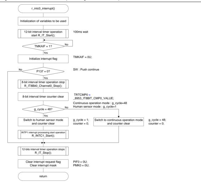
Figure 5.10 Processing INTP0 Interrupt
