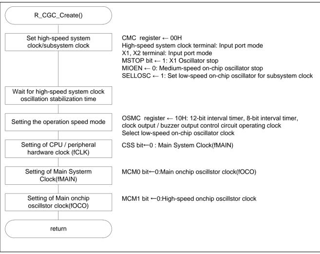
Figure 5.6 Clock Generator Setting
