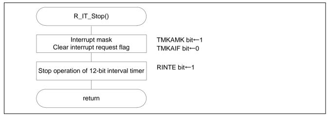
Figure 5.14 Stopping 12-Bit Interval Timer Operation
