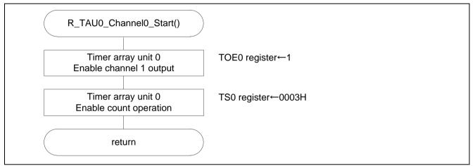
Figure 5.7 Starting Timer Array Unit 0 Operation
