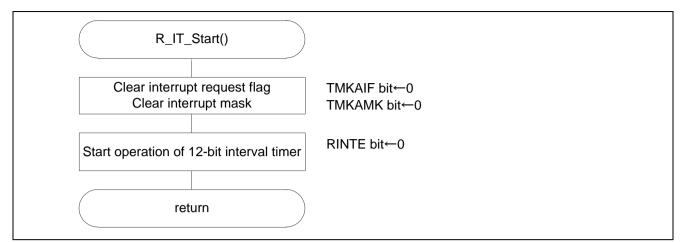
Figure 5.11 Starting 12-Bit Interval Timer Operation
