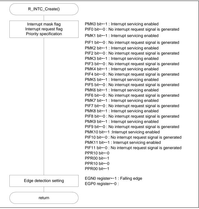
Figure 5.4 Setting External Interrupts
