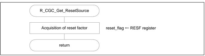
Figure 5.4 Acquisition of reset factor
