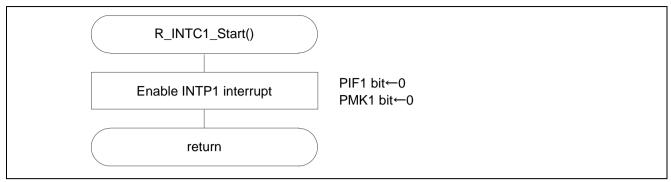
Figure 5.13 Starting INTP1 Interrupt Operation
