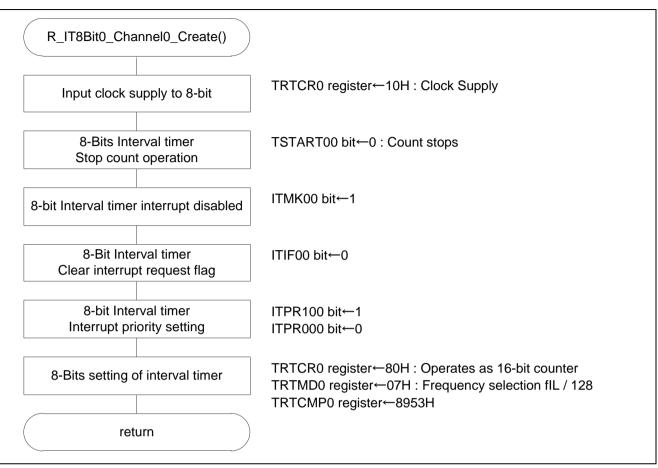
Figure 5.3 Setting 8-Bit Interval Timer
