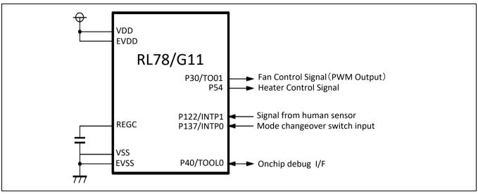
Figure 4.1 Hardware Configuration
