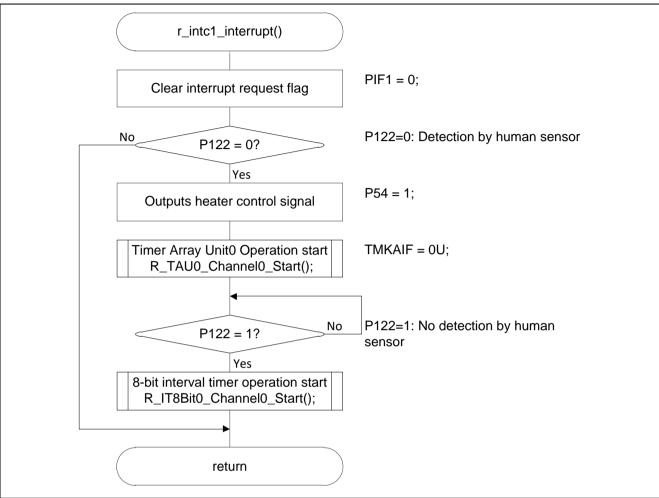
Figure 5.15 Processing INTP1 Interrupt
