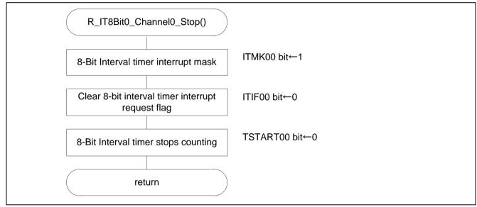
Figure 5.12 Stopping 8-Bit Interval Timer Operation
