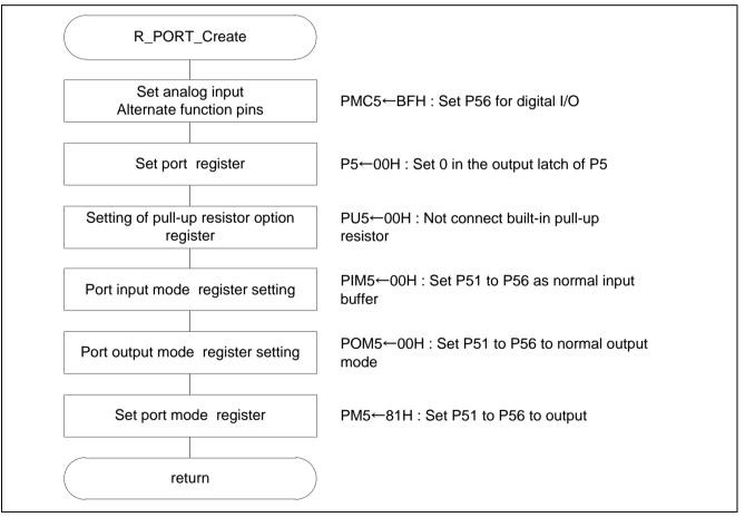
Figure 5.5 Input/Output Port Settings
