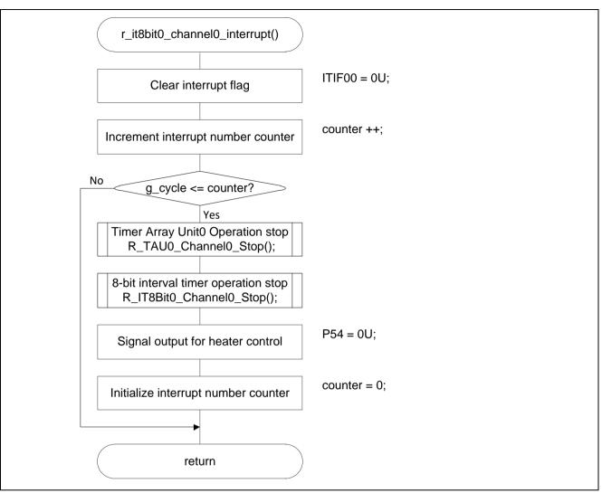
Figure 5.16 Processing 8-Bit Interval Timer Interrupt
