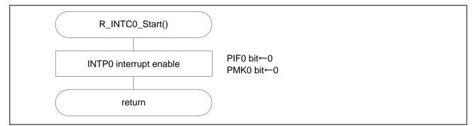
Figure 5.9 Starting INTP0 Interrupt Operation
