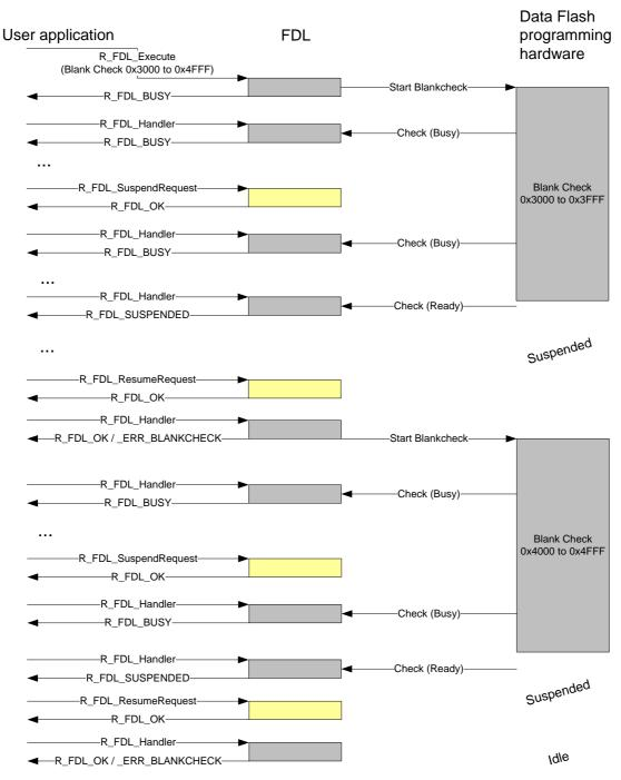
Figure 8: Suspend/Resume a blank check operation
