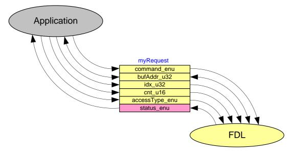
Figure 4: Usage of the request structure
