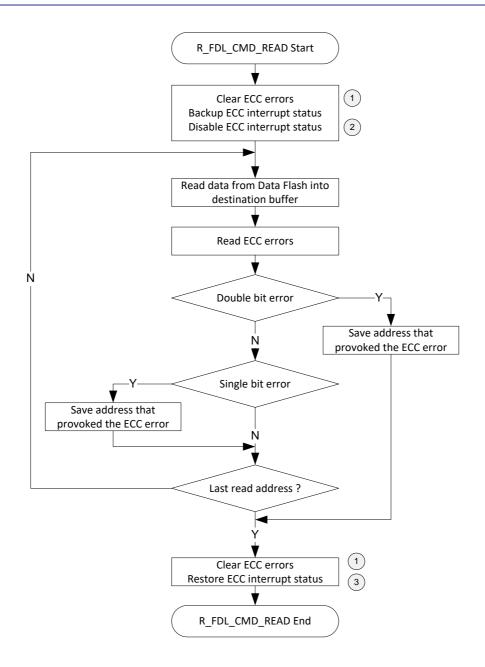
Figure 16: Handling of ECC error registers during read command
