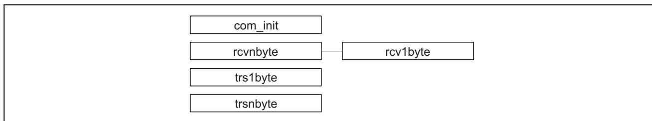
**Figure 21 Hierarchy of Asynchronous Serial Communication Program**
