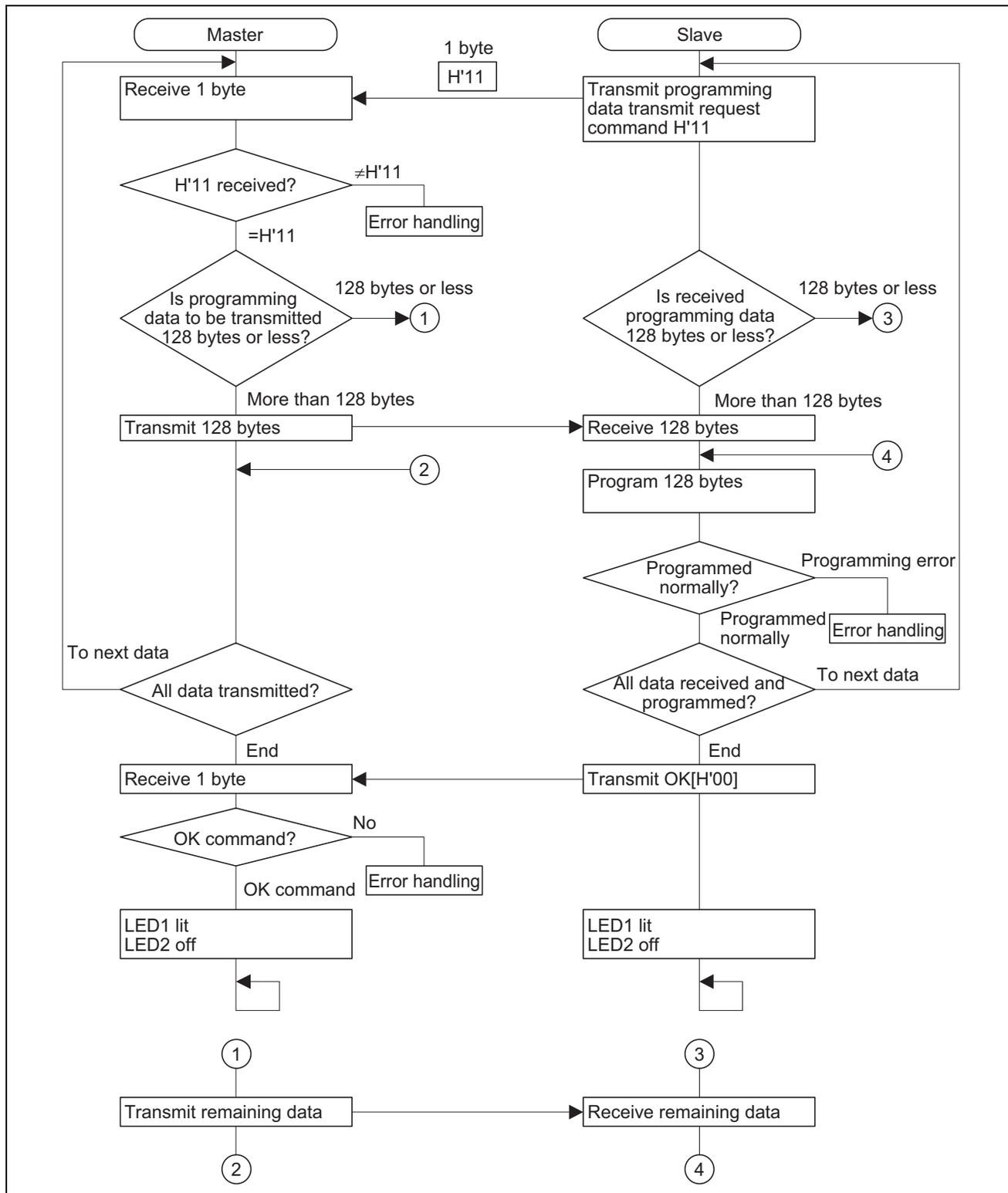
Figure 17 Programming Processing
