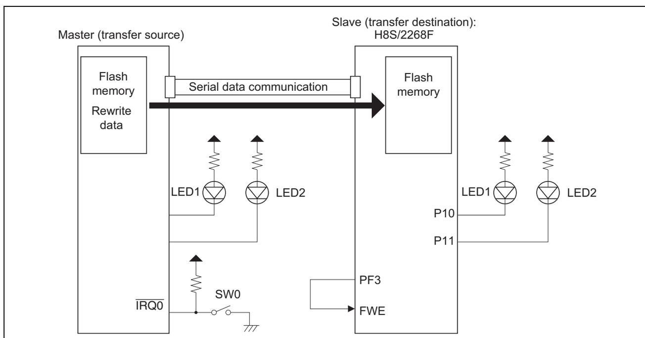
**Figure 1 Configuration Example of On-Board Rewrite Circuit**
