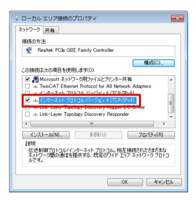
Select the IP address and subnet mask in the area indicated by the red frame in the figure below.
