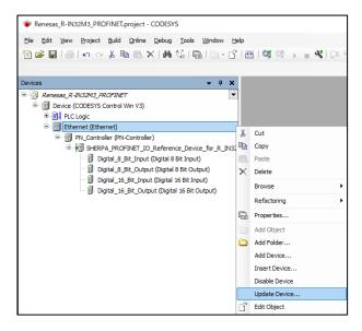
In the "Update Device" dialog box, select "Ethernet" under "Fieldbusses", "Profinet IO", "Ethernet Adapter", then click on the [Update Device] button.
