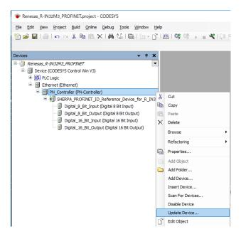
In the "Update Device" dialog box, select "PN\_Controller" under "Fieldbusses", "Profinet IO", "Profinet IO Master", then click on the [Update Device] button.
