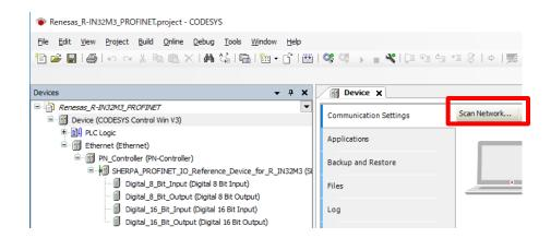
The "Select Device" window appears and a search for available devices that can use the local network automatically starts. The search is successful if a software PLC service is found. Double-click on the PC name displayed.
