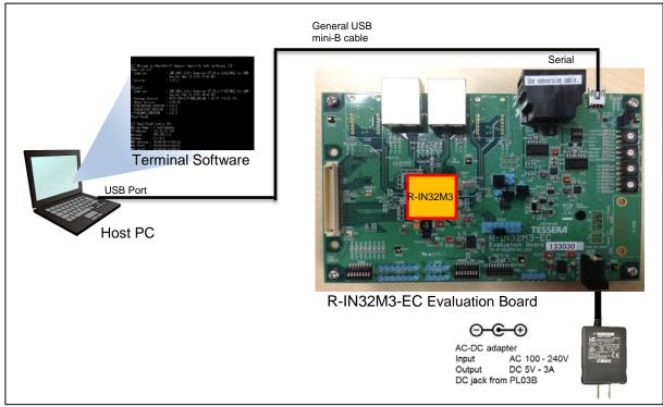
Figure A.1 System Configuration
