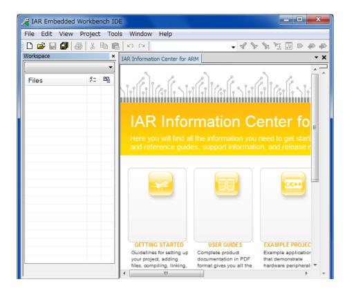
(2) Select [File]  $\rightarrow$  [Open]  $\rightarrow$  [Workspace] and double-click on the "rin32m3\_profinet.eww" filename in  $\pm$ an-r01an4282ej0100\_rin32m3\_profinet $\pm$ R-IN32M3\_PROFINET\_sample to open the workspace.
