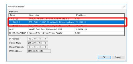
Check whether the IP address of the selected port has been correctly set.
