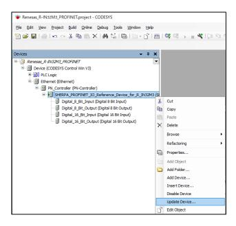
In the "Update Device" dialog box, select "SHERPA\_PROFINET\_IO\_Reference\_Device\_for\_R-IN32M3" under "Fieldbusses", "Profinet IO", "Profinet IO Slave", then click on the [Update Device] button.
