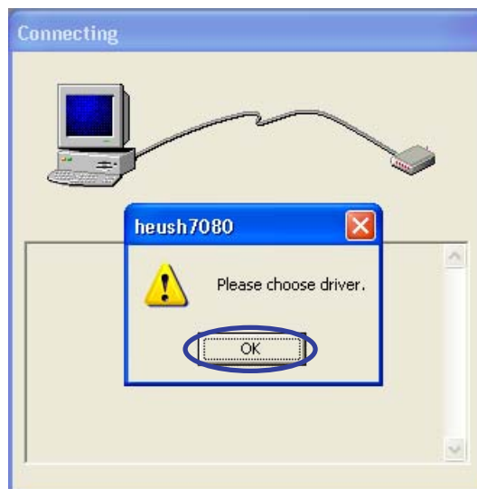
Figure 6.20 Prompt to Choose the Driver for the First-Time Connection of the E10A-USB Emulator
