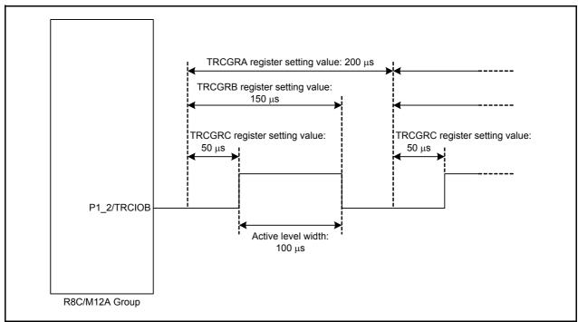
Figure 3.2 Timing Diagram
