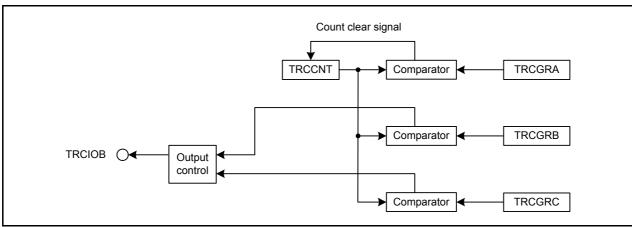
Figure 3.1 Block Diagram
