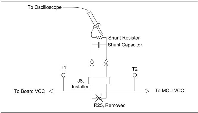
Figure 2. Configuration of current measurement with oscilloscope
