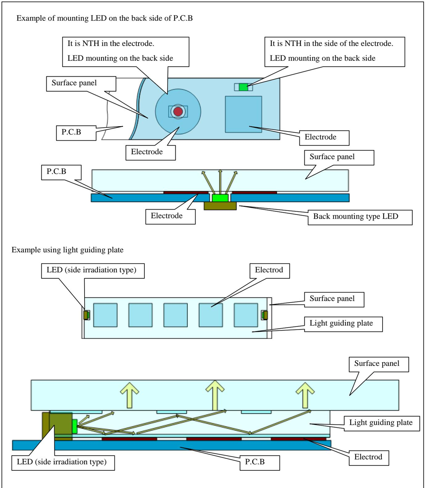
Figure 4-2 Example of arranging LED around touch electrode
