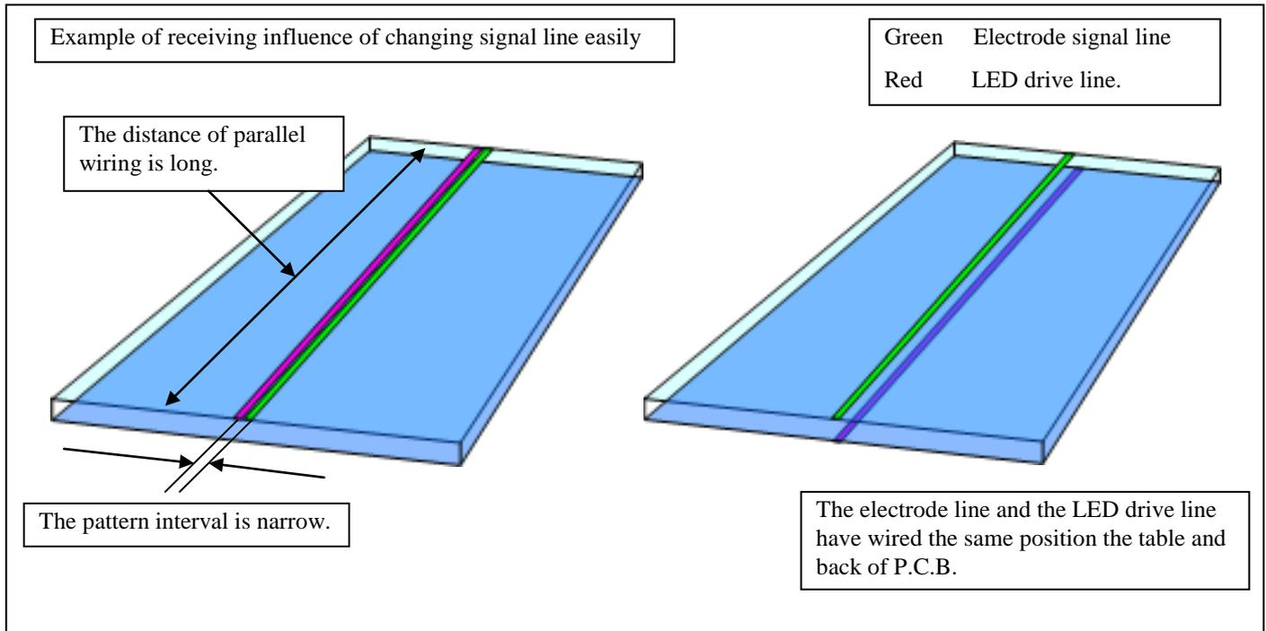
Figure 2-1 Example of LED drive line's influencing electrode signal line easily
