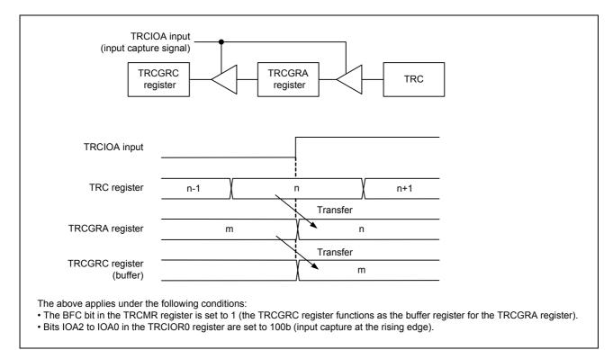
Figure 3.13 Buffer Operation for Input Capture Function
