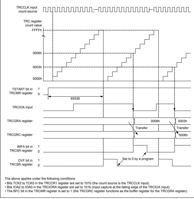
Figure 3.18 Operating Example of Input Capture Function
