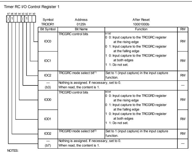
1. When the BFC bit in the TRCMR register is set to 1 (buffer register of TRCGRA register), set the IOC2 bit in the TRCIOR1 register to the same value as the IOA2 bit in the TRCIOR0 register.
