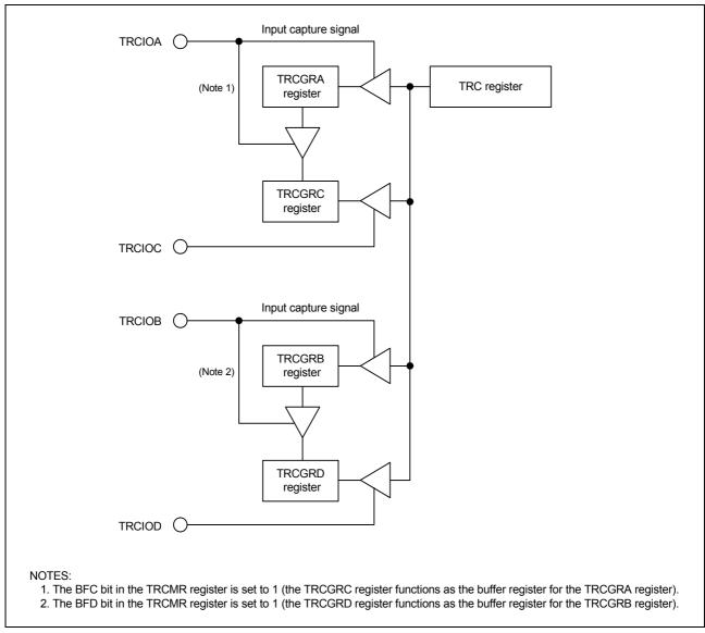
Figure 3.15 Block Diagram of Input Capture Function
