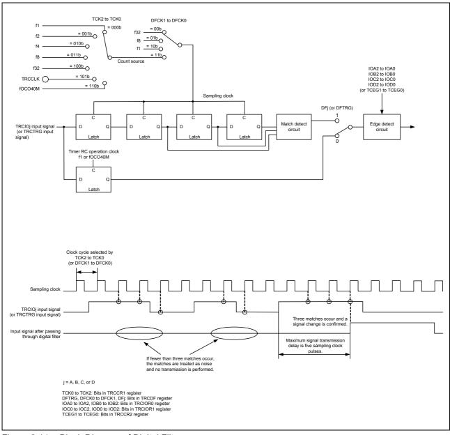
Figure 3.14 Block Diagram of Digital Filter
