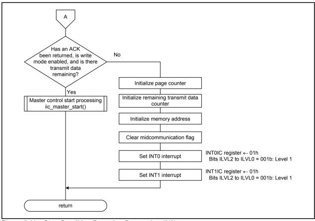
Figure 5.11 Stop Condition Detection Processing (2/2)
