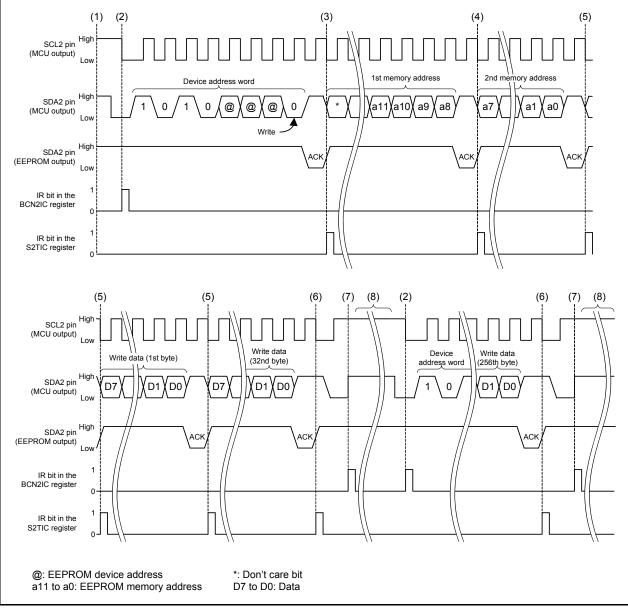
Figure 5.1 shows the Timing Diagram in Write Mode.
