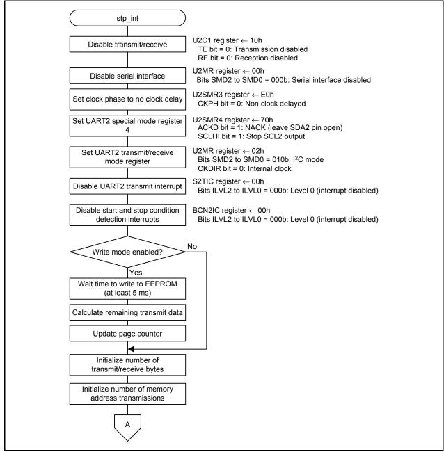
Figure 5.10 Stop Condition Detection Processing (1/2)
