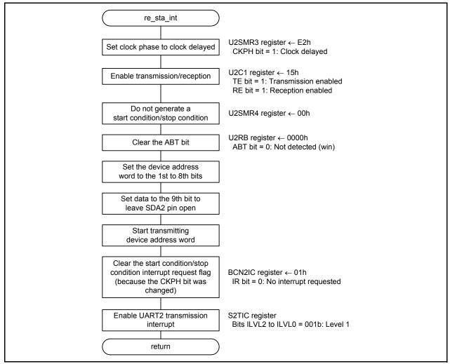
Figure 5.12 Restart Condition Detection Processing
