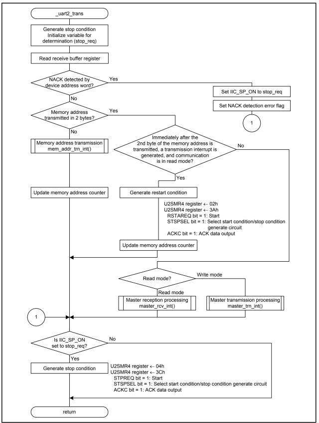
Figure 5.13 UART2 Transmit Interrupt Handling
