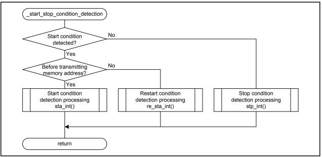
Figure 5.8 Start Condition/Stop Condition Detection Interrupt Handling
