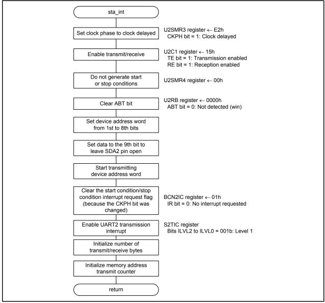
Figure 5.9 Start Condition Detection Processing
