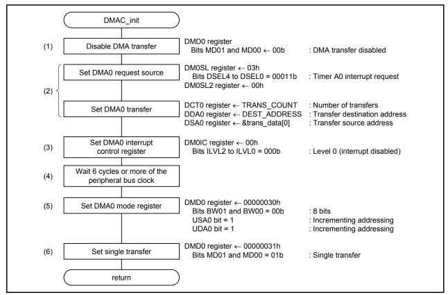
Figure 4.4 DMAC Initial Setting
