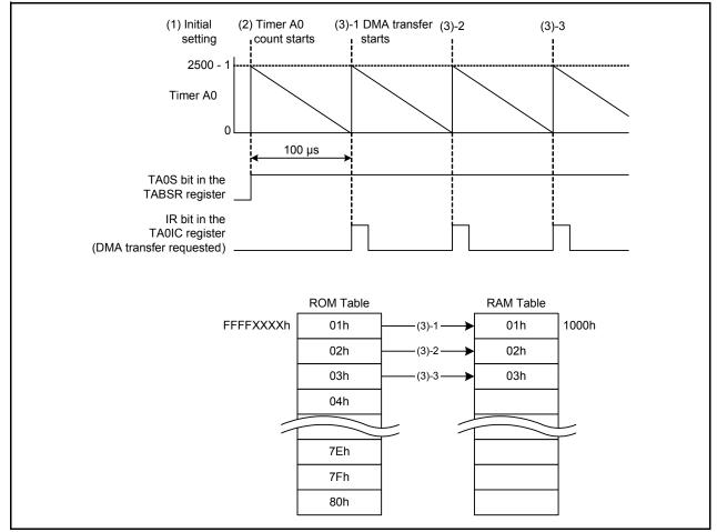
Figure 4.1 Timing Diagram
