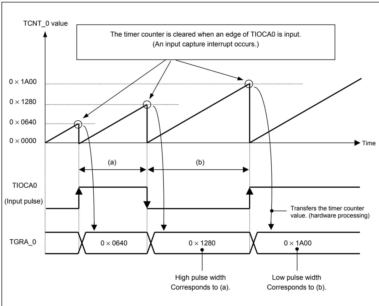
Figure 2 Example of Pulse Width Measurement
