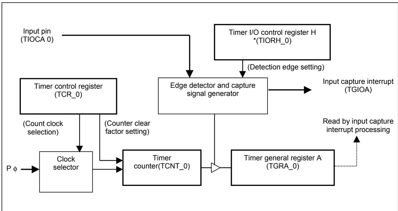
Figure 1 Block Diagram of Pulse Width Measurement
