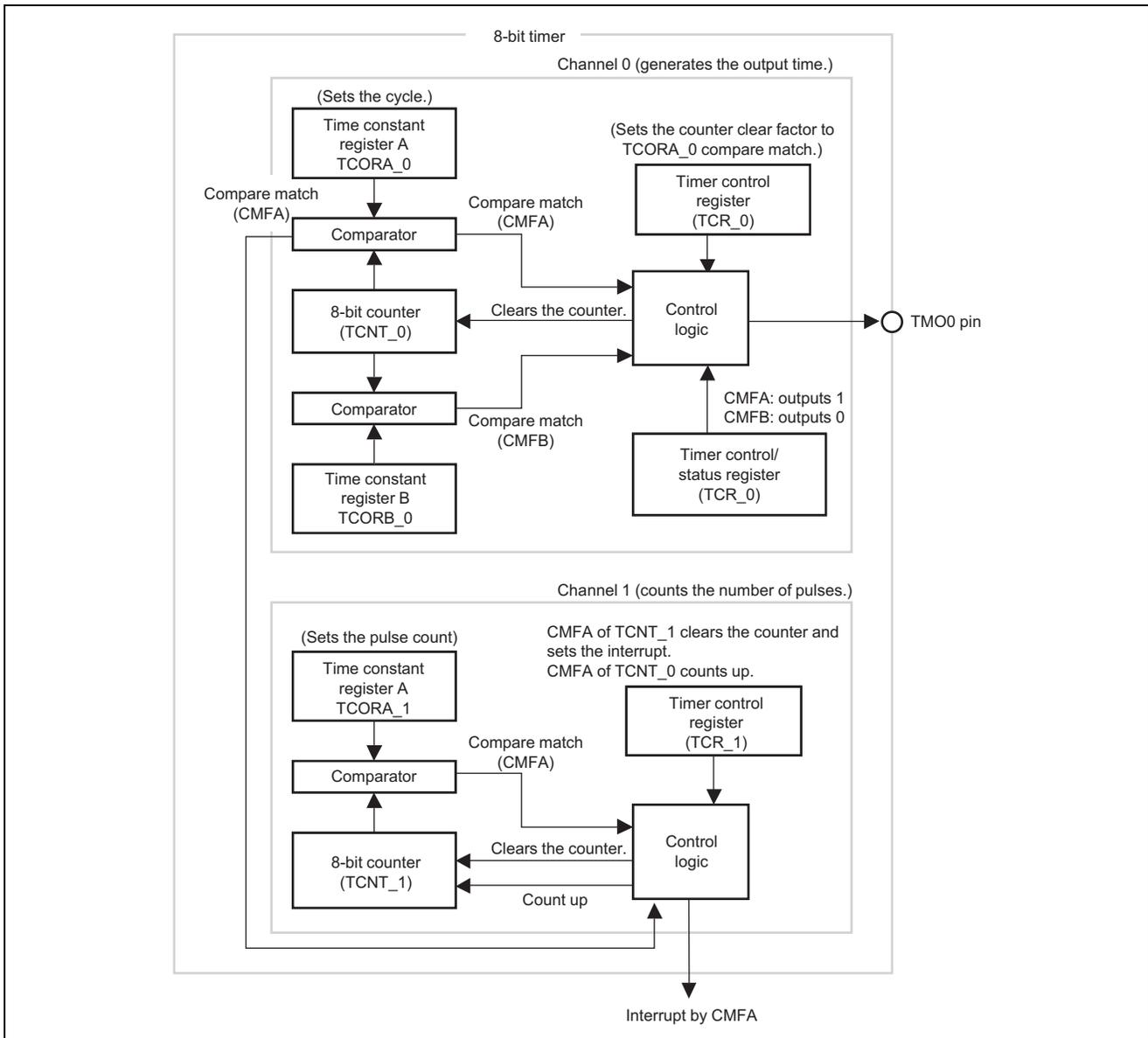
Figure 2 Block Diagram of Output Pulse Count
