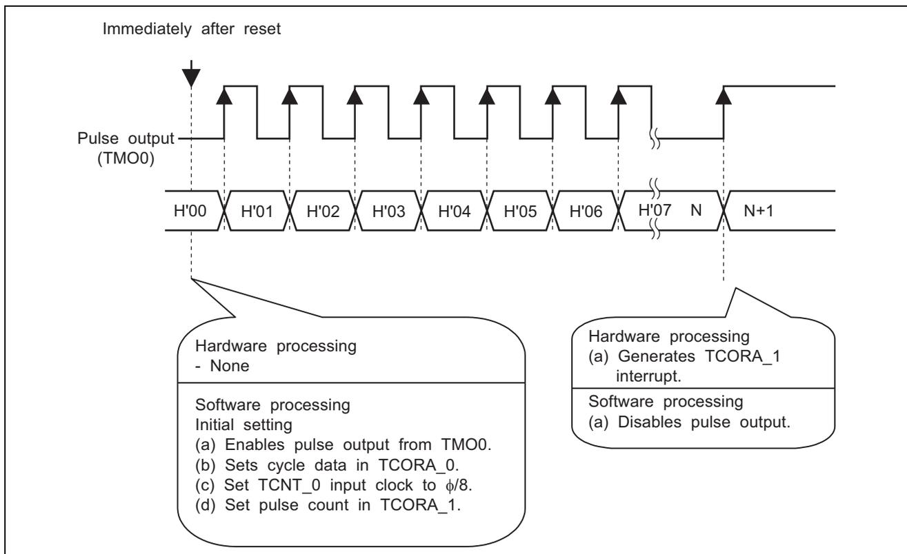
**Figure 3 Description of Operation of Pulse Output**
