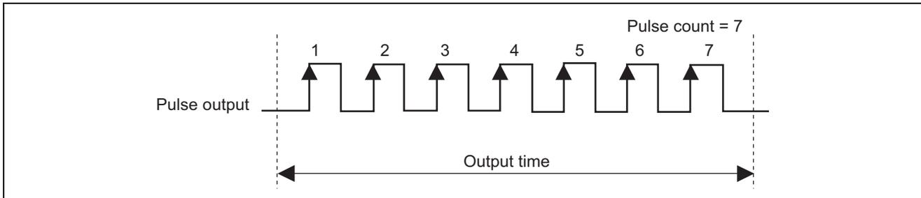
**Figure 1 Pulse Output Timing**
