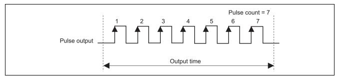
Figure 1 Pulse Output Timing
