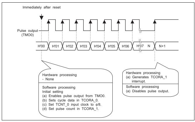
Figure 3 Description of Operation of Pulse Output
