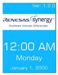
2. Tap the splash screen to enter the Thermostat demo. In this demonstration, the SSP uses the A/D converter to read the internal temperature sensor of the S5D9 and display this information on the LCD Display.
