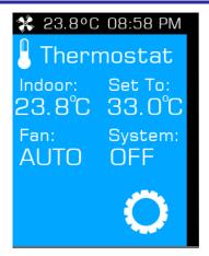
3. Tap the settings icon (looks like a gear) on the bottom right to make adjustments to the system including Units, Time and Date.
