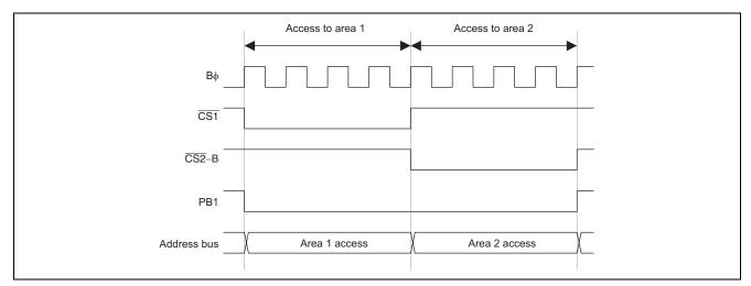
Figure 4 Timing when Multiple  $\overline{\text{CS}}$  Signals are Output through a Single Pin
