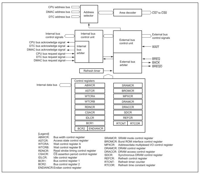
Figure 2 Block Diagram of the Bus Controller
