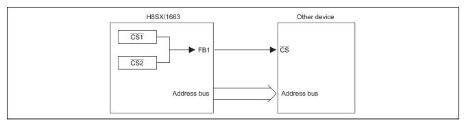
Figure 1 Example of Connection for Output of Multiple CS Signals through the Same Pin
