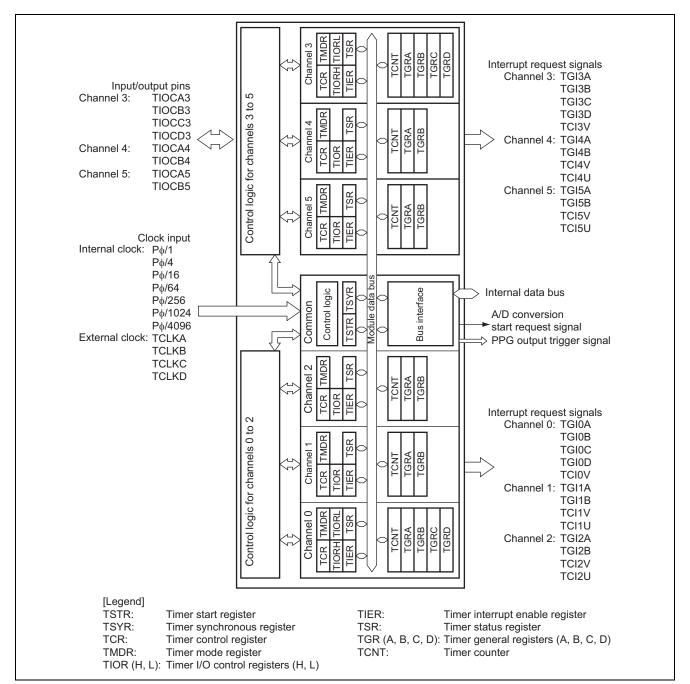
Figure 2 Block Diagram of the TPU
