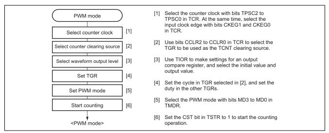
Figure 4 Example of Procedure for Setting PWM Mode
