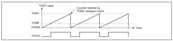
Figure 5 Example of PWM Mode Operation (1)
