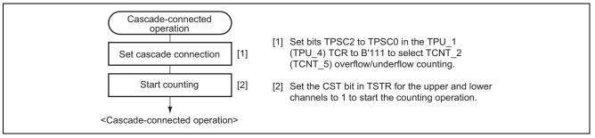
Figure 3 Example of Procedure for Setting Cascade-Connected Operation
