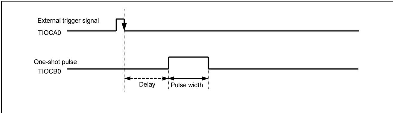
Figure 2 Example of One-Shot Pulse Output
