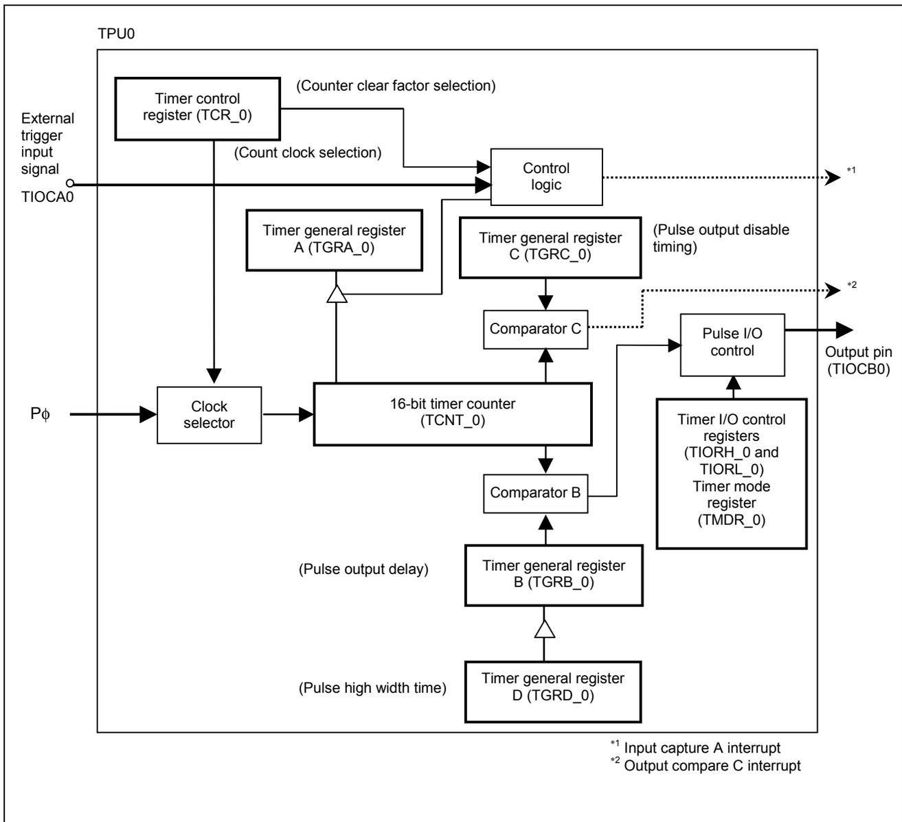
Figure 1 Block Diagram of One-Shot Pulse Output
