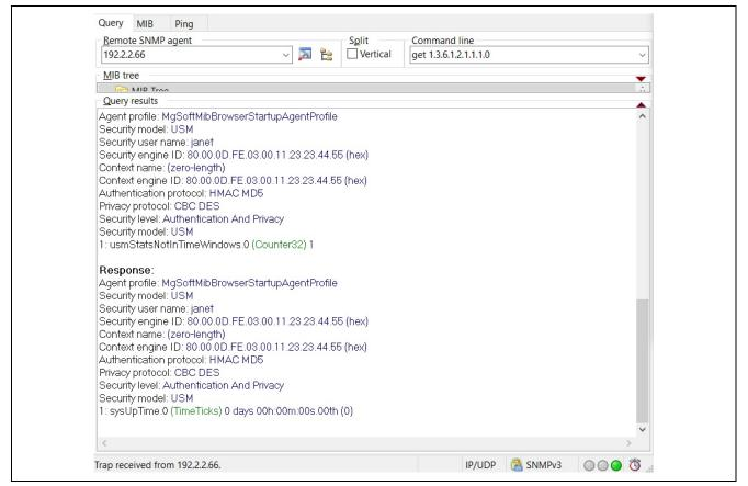
Figure 10 Log capture of SNMP Manager 'handshake' with NetX Duo SNMP Agent Project from the MG-Soft MIB Browser application
