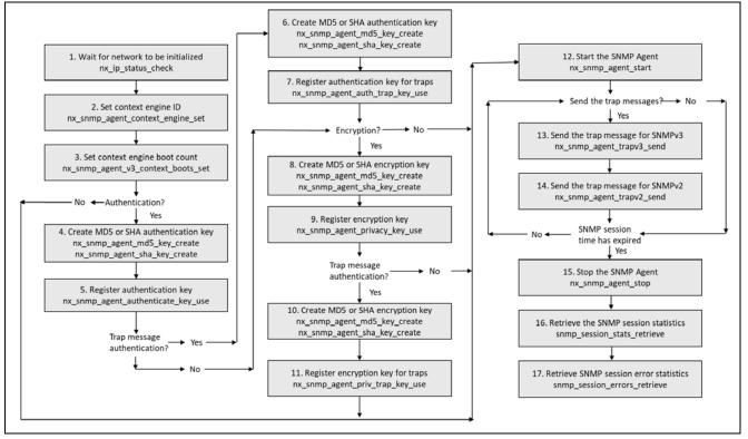
Figure 8 NetX Duo SNMP Agent Application Project Flow Diagram
