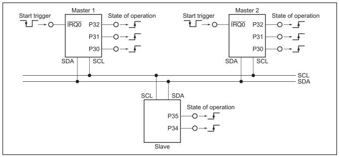
Figure 1 Connections for I<sup>2</sup>C Bus Interface 2 Multi-Master Mode Communication
