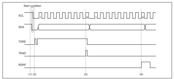
Figure 3 Timing of Operations in Master Receive Mode 1
