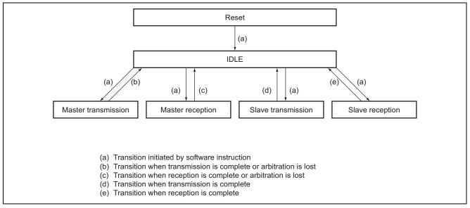
Figure 7 State Transition Diagram
