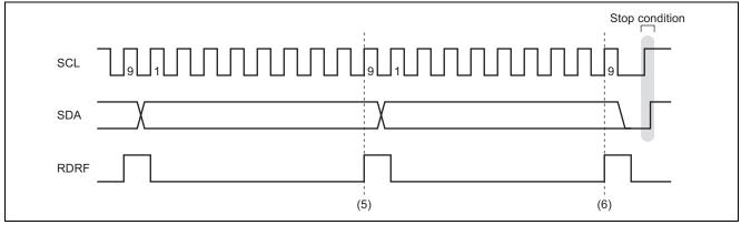
Figure 4 Timing of Operations in Master Receive Mode 2
