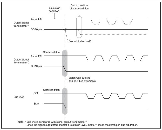
Figure 5 Loss of Bus Arbitration when the Start Condition is Detected
